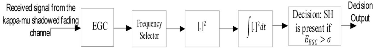
Fig. 1: Block diagram of local sensing using ED with EGC
