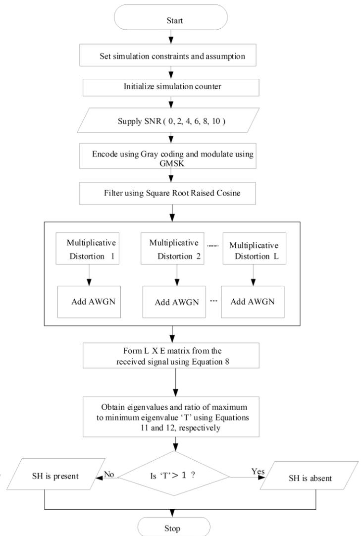
Fig. 3b: Flowchart for Detecting SH using EVD
