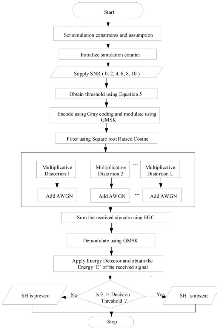
Figure 3a: Flowchart for Detecting SH using ED
