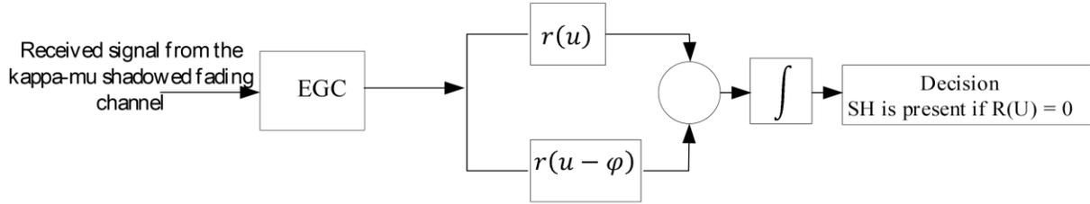
Fig. 2: Block diagram of local sensing using CD with EGC
