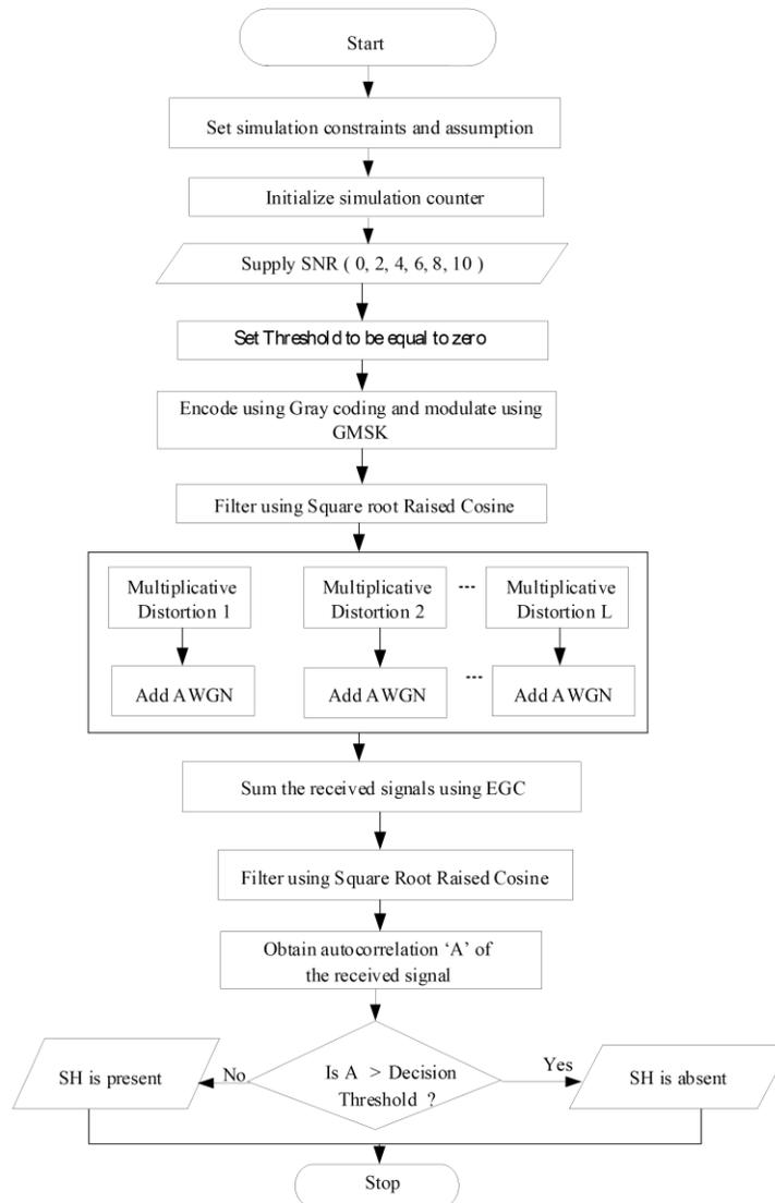
Figure 3c: Flowchart for Detecting SH using CD
