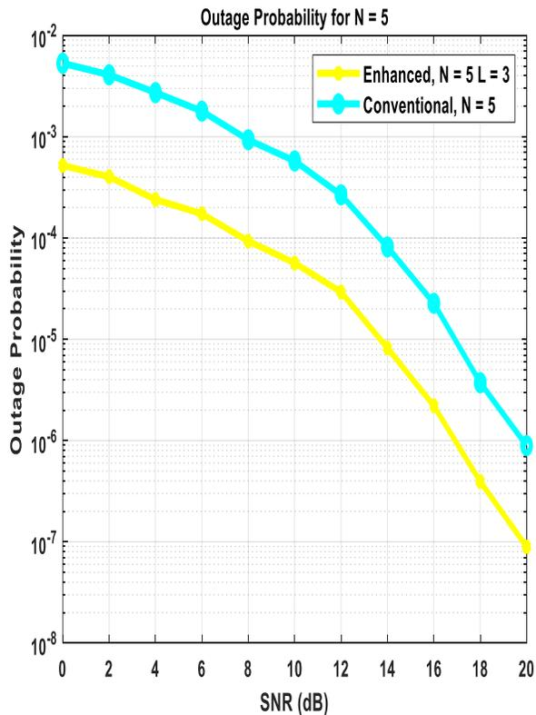
Figure 5:  $P_{out}$  versus SNR for enhanced and conventional technique at N=5 and L=3.
