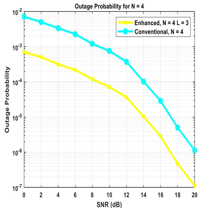
Figure 3:  $P_{out}$  versus SNR for enhanced and conventional technique at  $N=4$  and  $L=3$ .
