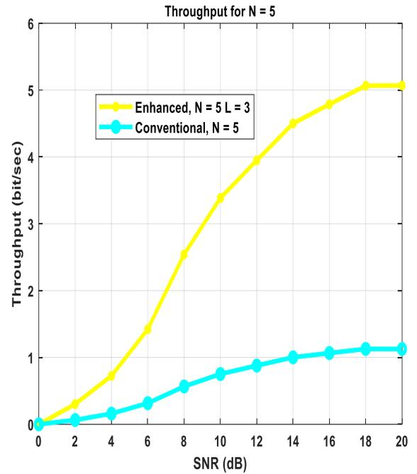
Figure 6: Throughput versus SNR for enhanced and conventional technique at N=5 and L=3.
