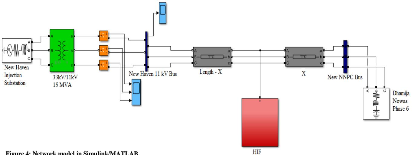
Figure 4: Network model in Simulink/MATLAB.
