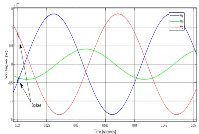
**Figure 9: System voltage showing voltage spikes.**
