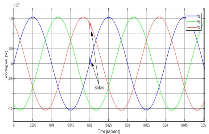
Figure 6: System voltage showing spikes.
