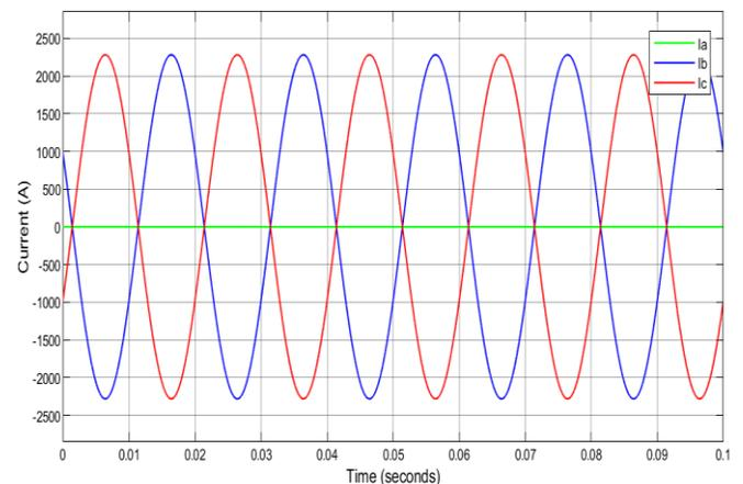
**Figure 11: System phase A, B and C currents during HIF.**
