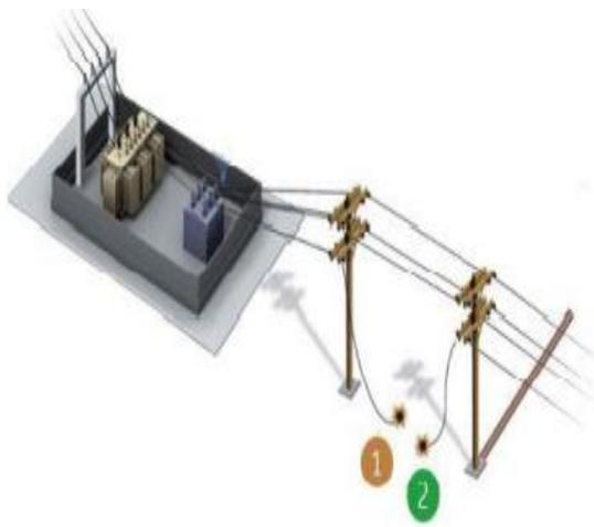
**Figure 1: Source-end and load-end downed conductors on asphalt surface (Theron *et al.*, 2018)**
