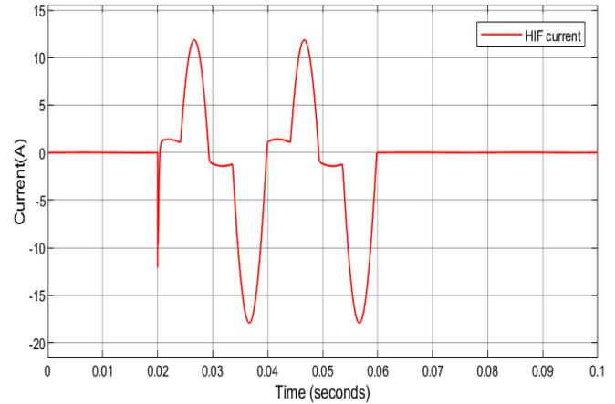
Figure 5: High impedance fault current on phase A-G.
