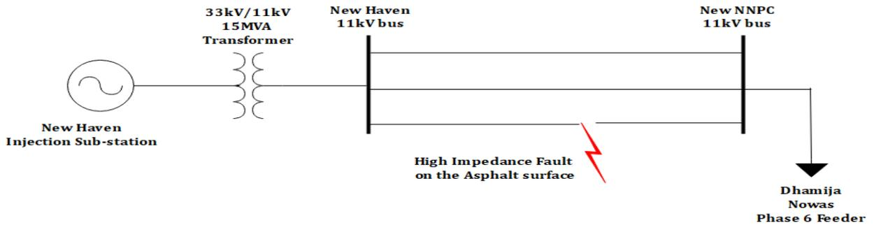
Figure 3: Detailed schematic network for the analysis.
