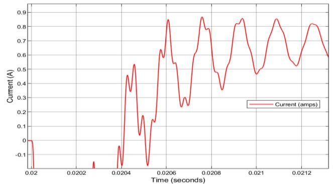
**Figure 10: Transformer neutral current during HIF.**
