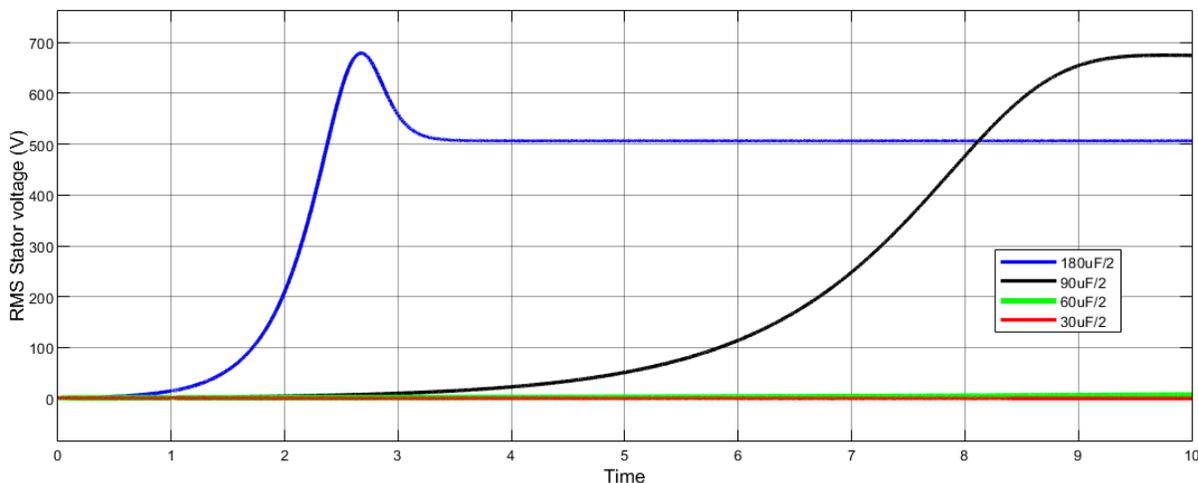
Figure 11: Voltage behavior of SEIG under different excitation capacitance at 200 rad/sec.
