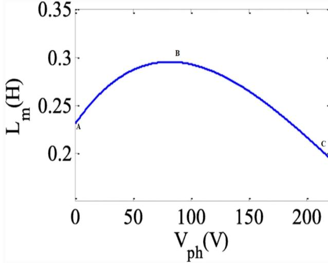
Figure 3: Saturation curve of Induction generator (Bendjeddu *et al.*, 2021).
