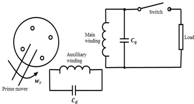
Figure 1: Schematic diagram of a capacitive excited and self-regulated induction single-phase generator.
