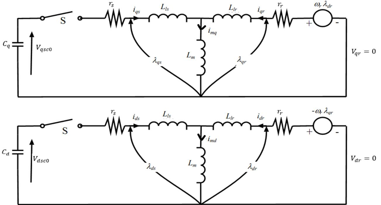
Figure 5: Equivalent circuit of capacitive SEIG.
