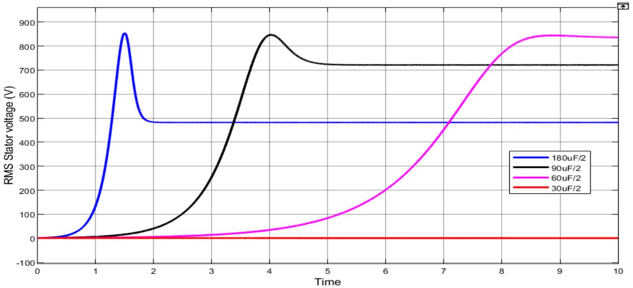
Figure 10: Voltage behavior of the SEIG under different excitation capacitance at 250 rad/sec.
