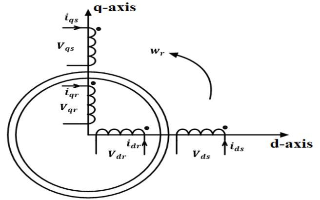
Figure 4: d-q representation of induction machine.
