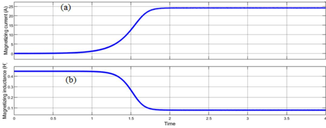
Figure 8: (a) Magnetizing current (b) Magnetizing inductance.
