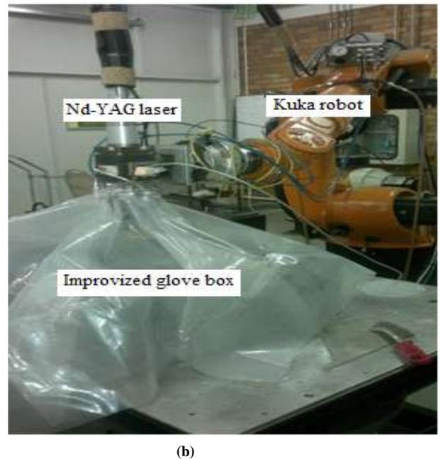
**Figure 1. (a) Schematic of the LMD process (Mahamood et al. 2013) (b) Pictorial diagram of the experimental set-up.**
