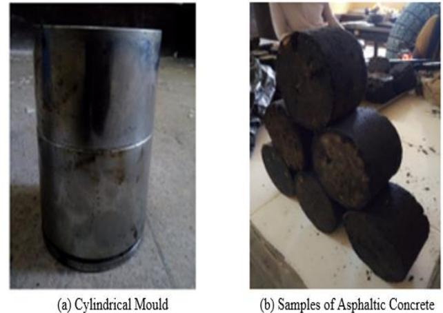
**Figure 2:** Cylindrical mould and asphaltic concrete samples.
