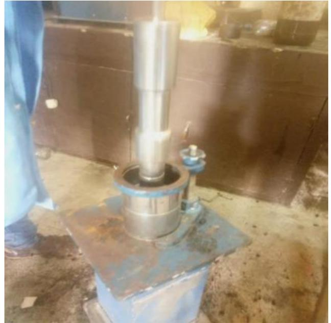
Figure 3: Sample of Asphalt concrete in the compaction mould.
