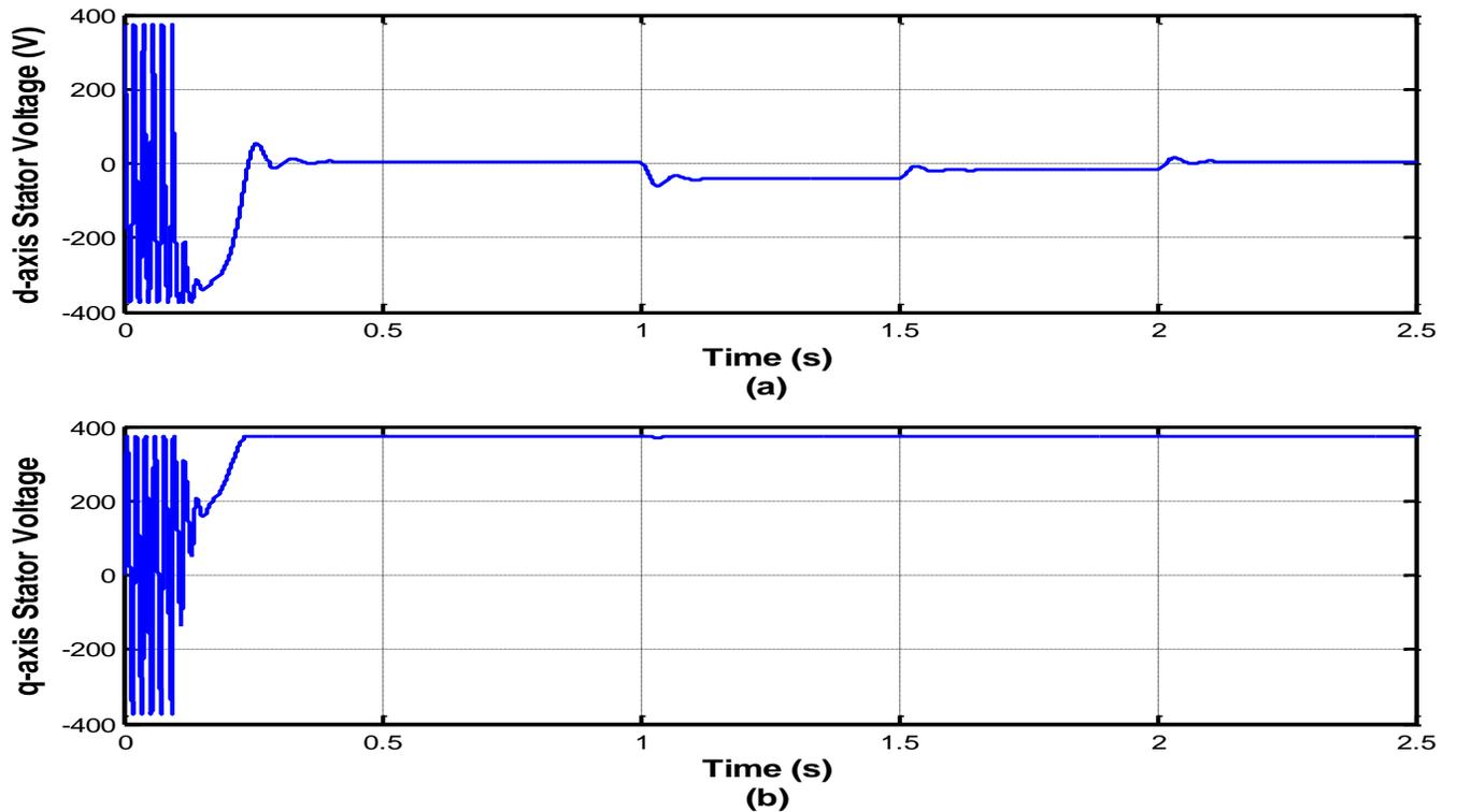
Figure 7: Direct and quadrature axis voltages in the stator.
