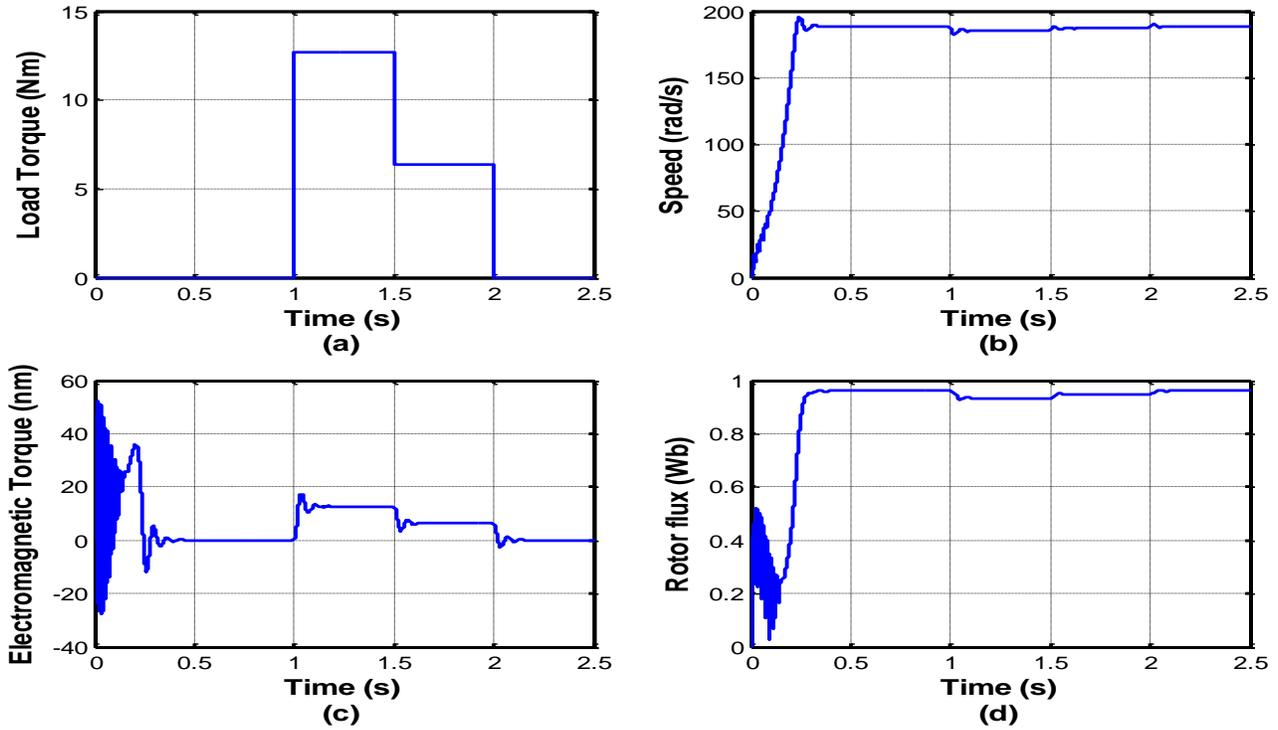
Figure 4: Simulation results of the motor behavior (a) Load torque with Time (b) Speed with Time (c) Electromagnetic torque with Time (d) Rotor flux with Time.
