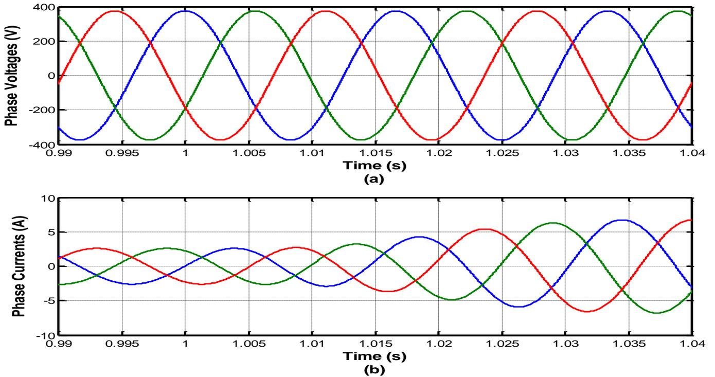
Figure 5: Simulation results of stator phase voltages and currents.
