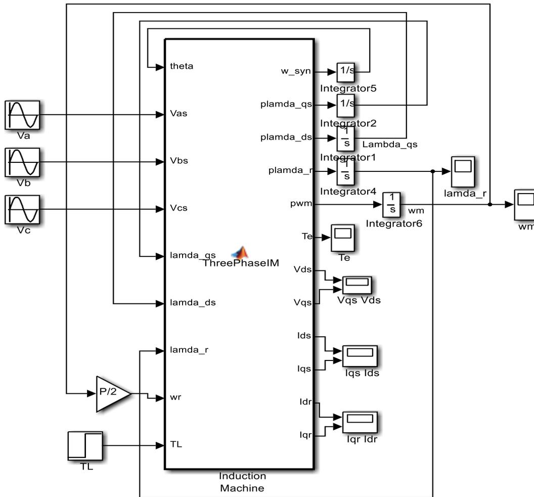
Figure 3: MATLAB/Simulink block to implement the solution diagram.
