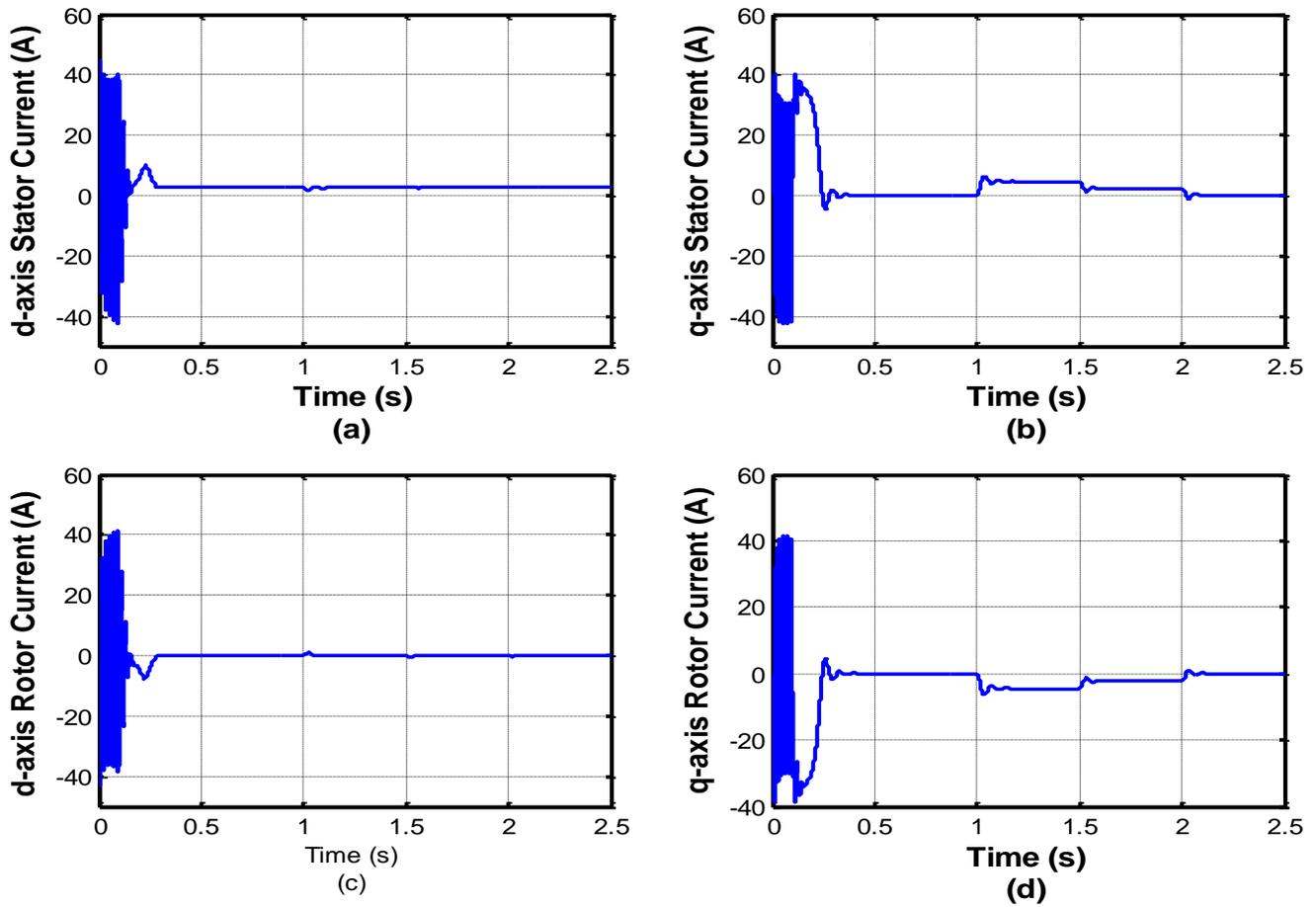
Figure 6: Simulation results of  $d$  and  $q$ -axis stator and rotor currents.
