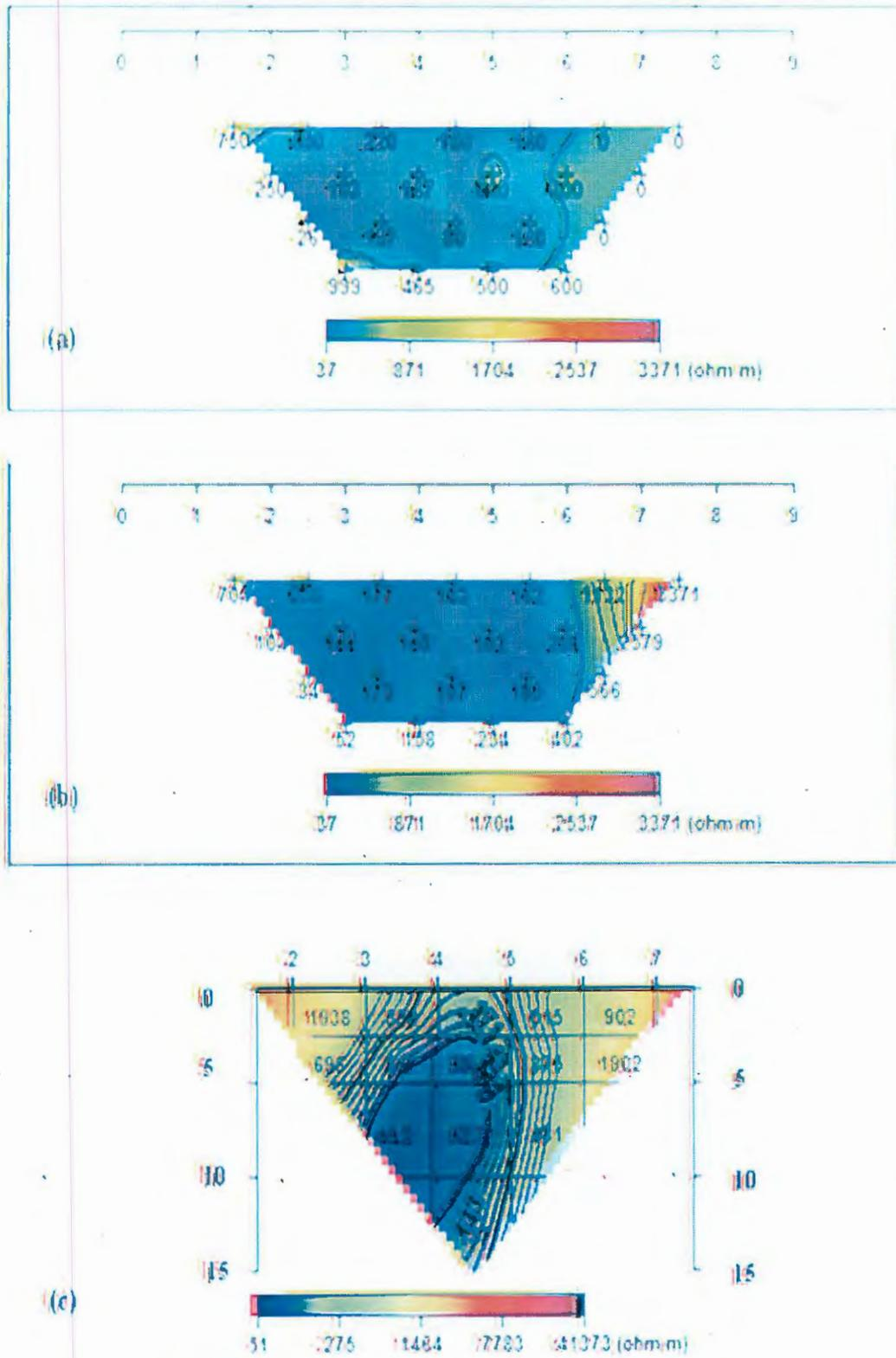
**Fig. 4: (a) Field data pseudosection, (b) Theoretical data pseudosection and (c) 2-D resistivity structure along traverse AB.**
