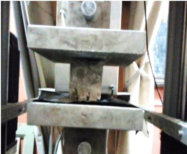
Figure 2: Determination of compressive strength of the concrete.
