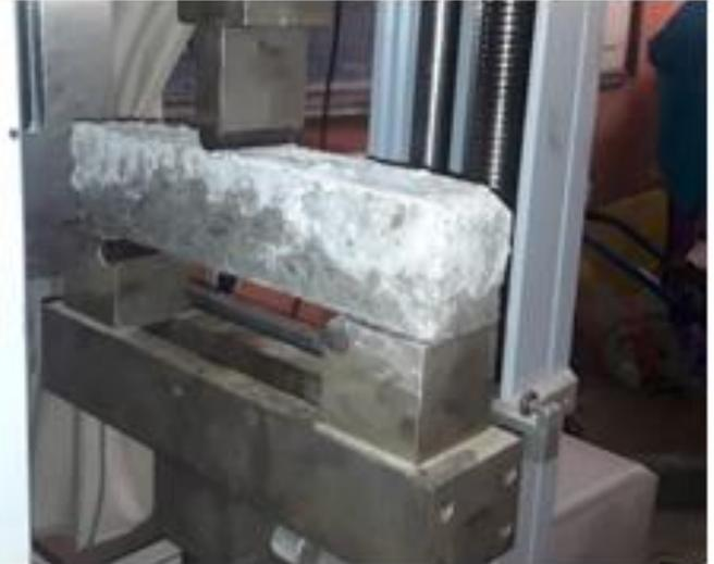
Figure 3: Determination of flexural strength of the concrete.
