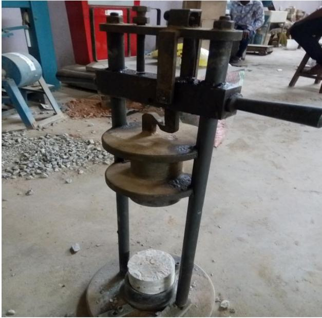
Figure 5: Aggregate impact testing machine.
