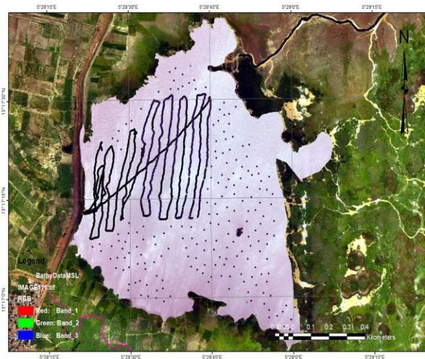
Figure 5: The extent of bathymetry survey over Lugu dam reservoir.
