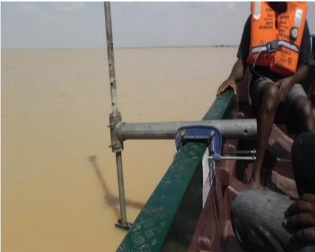
Figure 2: Echo sounder attached to the flying boat during data acquisition.
