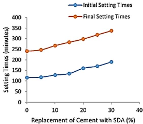
Figure 4: Initial and final setting times of paste with SDA (Elinwa & Ejeh, 2004.).
