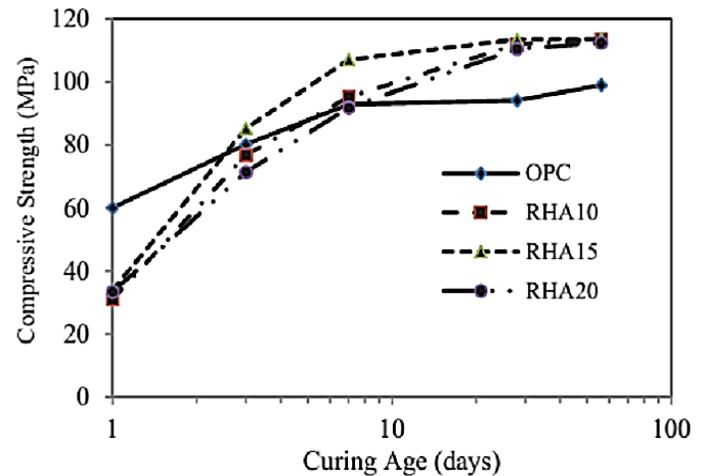
Figure 2: Effect of RHA on the compressive strength of concrete (Mahmud *et al.*, 2016).
