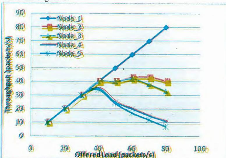
**Figure 6: The Effect of Bottleneck Collision Domain on the Network Capacity**
