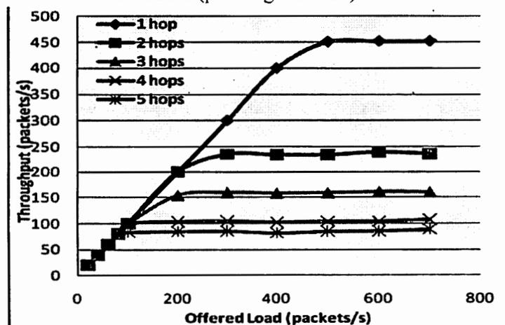
**Figure 4: Effect of Mesh Forwarding on Wireless Mesh Network Capacity**
