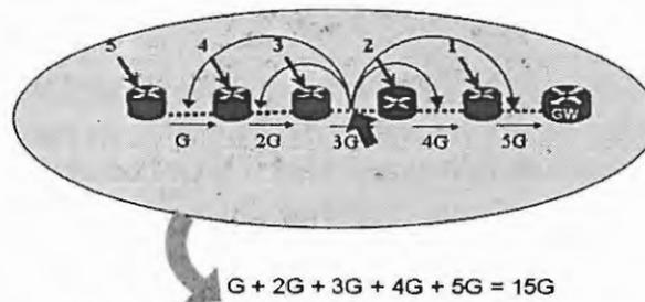
**Figure 5: A Linear Wireless Mesh Network Scenario to Analyse the Effect of Bottleneck Collision Domain on the Network Capacity**
