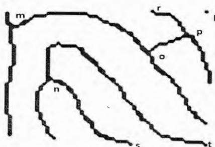
Fig. 7b. Thinning using only the Zhang-Suen's algorithm
