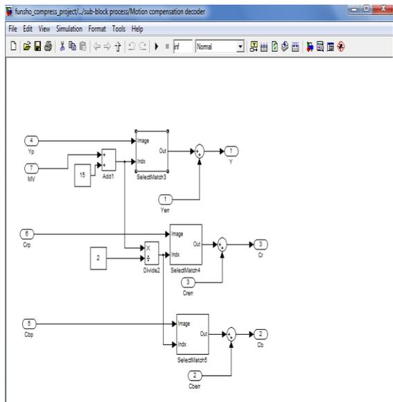
Figure 4: Motion Compensation/Estimation Block.
