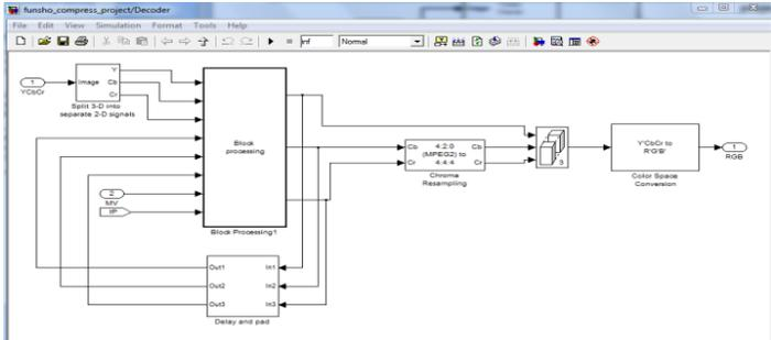
Figure 3: Block Process for the Video Compression (Decoder Block)
