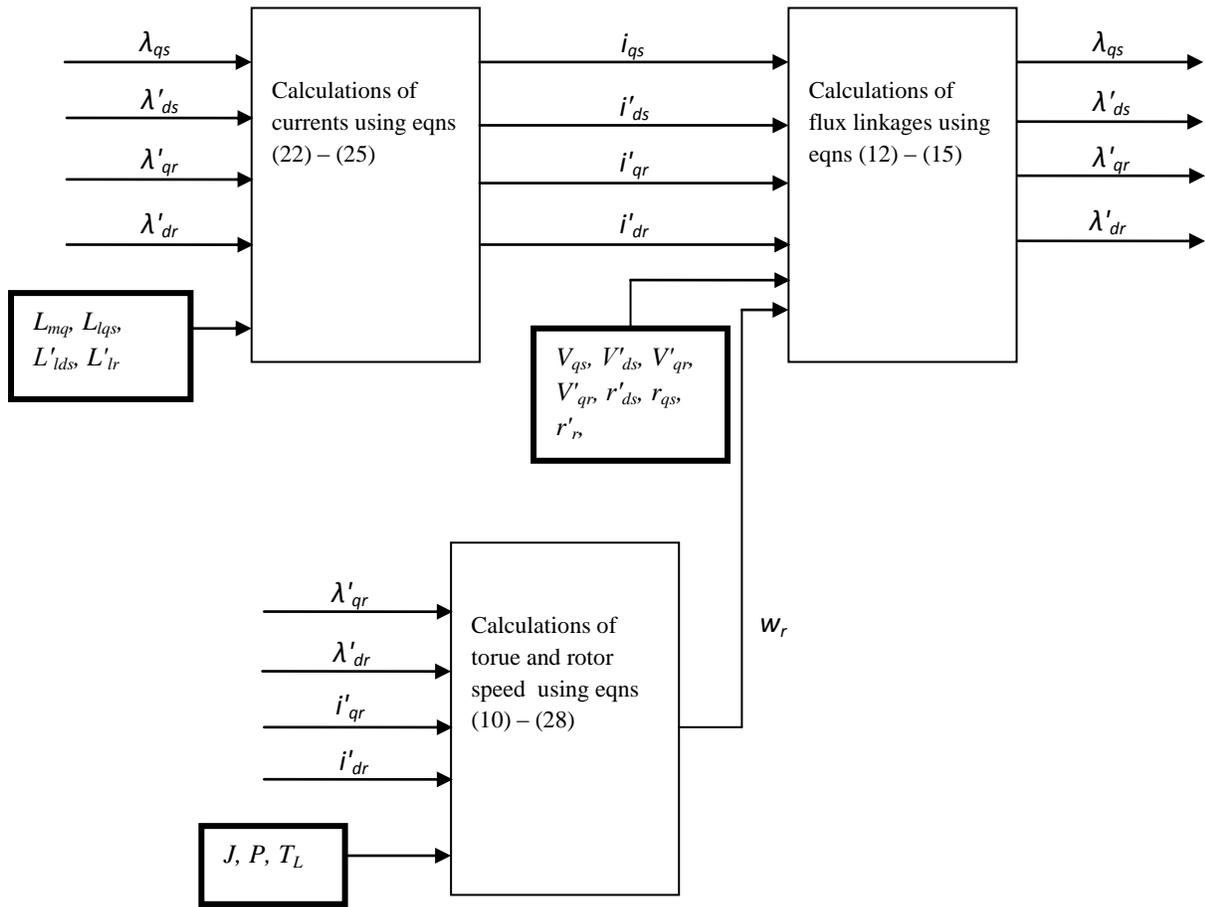
Figure A1: Block Diagram of the solution of model equations
