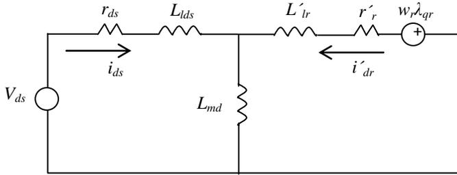
Figure 2(b): d-axis equivalent circuit of the machine
