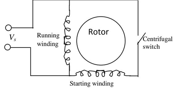
Figure 1: Schematic diagram of the Split-Phase Induction Motor
