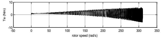
Figure 11: Dynamic torque-speed characteristics of the machine
