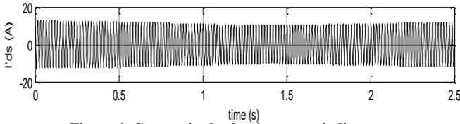
Figure 6: Current in the d-axis stator winding
