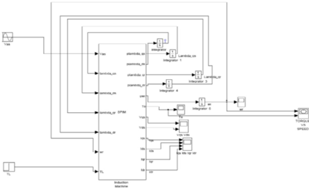
Figure A2: Simulink model of the split phase induction machine
