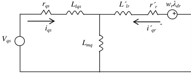
Figure 2(a): q-axis equivalent circuit of the machine
