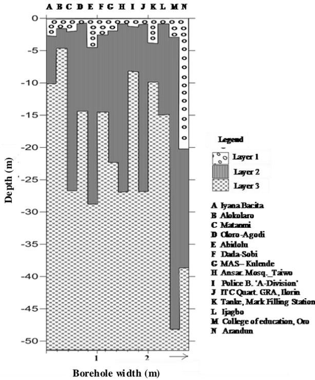
Figure 8 Lithological section of boreholes within the study area (N S)
