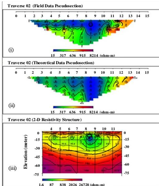
Figure 5b: (i) Field data pseudosection (ii) Theoretical data pseudosection and (iii) 2-D resistivity structure along traverse 02
