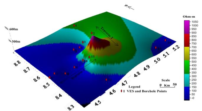
Figure 7: Apparent resistivity 3-D surface for AB/2 equals 50m within the study area
