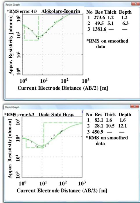
Figure 4a: Typical Schlumberger sounding curves obtained in the study area
