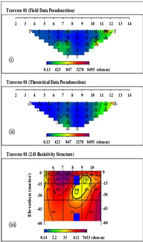
Figure 5a: (i) Field data pseudosection (ii) Theoretical data pseudosection and (iii) 2-D resistivity structure along traverse 01
