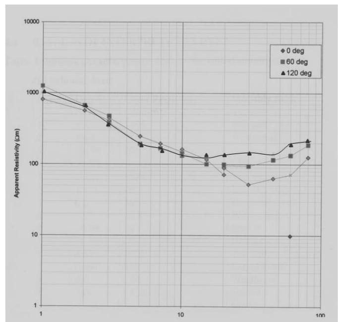
**Figure 5: VES sounding curve of radial sounding (at 0°, 60° and 120°).**
