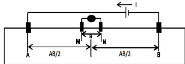
Figure 2: A schematic representation of the Schlumberger array.
