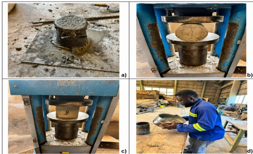
Figure 1 Material preparation for specimen casting: (a) slump test, (b) compressive test of cylinder, (c) compressive test of cube, (d) aggregate sieving.
