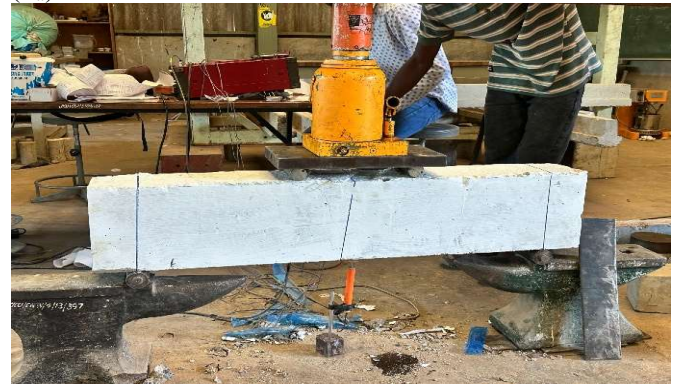
Figure 3. Four-point bending test setup showing all instruments including the LVDT, load cell, and hydraulic jack.
