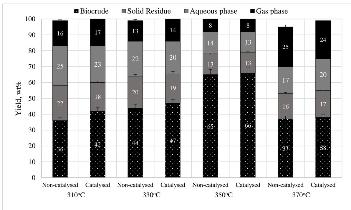
Figure 1: Products derived from HTL of microalgae with and without catalyst at different reaction temperature.
