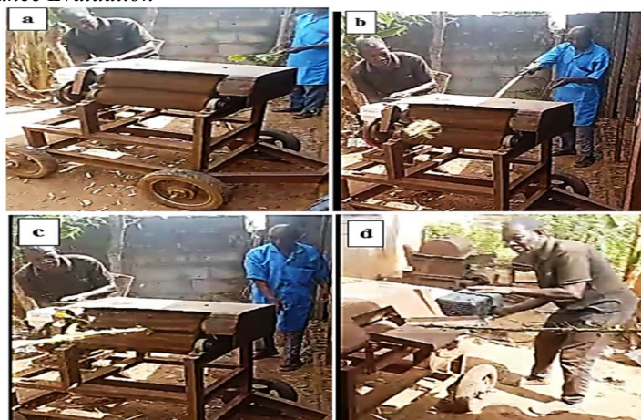
Figure 8 Experiment procedure, a. Inserting kenaf stem, b. Decortication ongoing, c. Decorticated kenaf stem, d. adjusting engine speed
