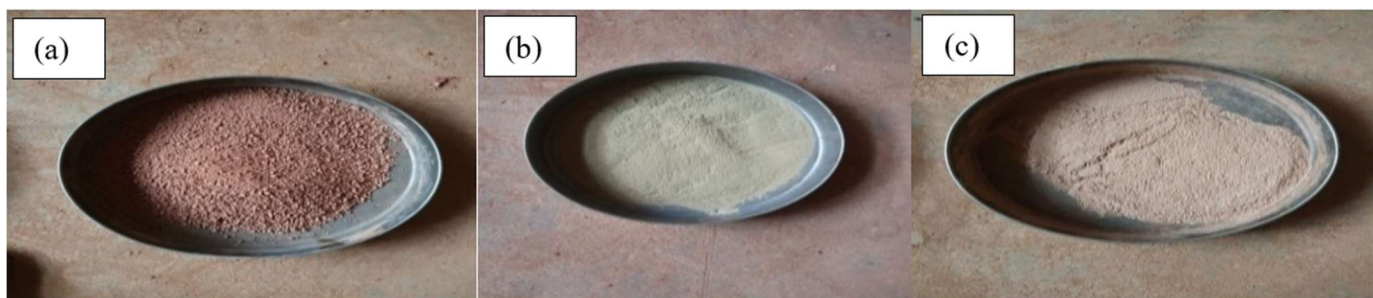
Figure 1 Constituent materials (a) Pulverized lateritic soil (b) Bentonite (c) Ceramic Dust
