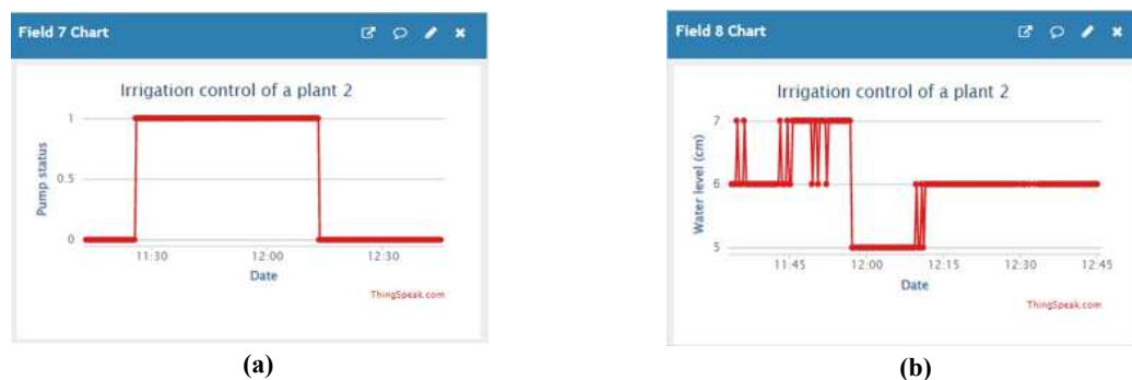
Figure 24 ThingSpeak Charts of Pump Status and Water Tank Level: a) Pump Status; b) Water Tank Level.
