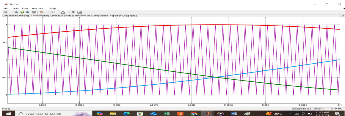
Figure 14 Pulse modulated signal using TPWM (triangular PWM)
