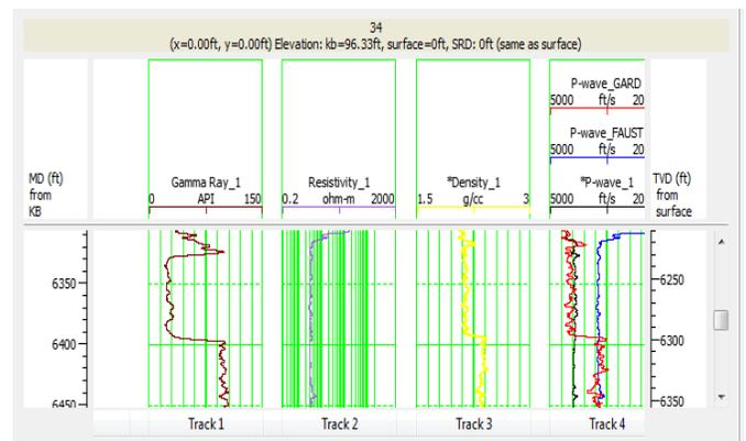
Figure 2: Log display of acquired P-Wave log (black curve), P-wave derived from Gardner (red curve) and Faust methods (blue curve) in tract 4.
