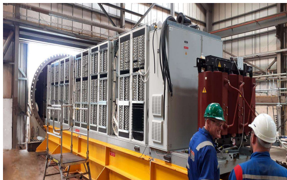
Figure 1 Rack Payload comprising servers in the Microsoft Underwater Datacentre developed by Naval Group. Source: (Naval Group, 2020).
