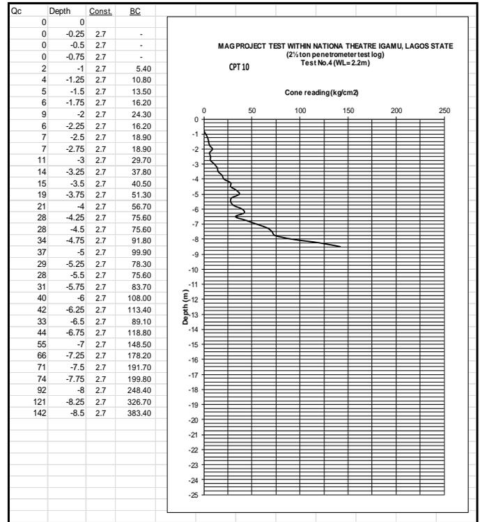
Figure 5d: Selected cone resistance versus depth curve at test point 10.
