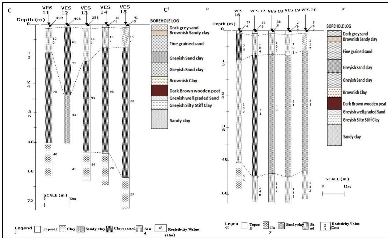
Figure 3: Geo-electric Section along CC<sup>1</sup> and DD<sup>1</sup>.
