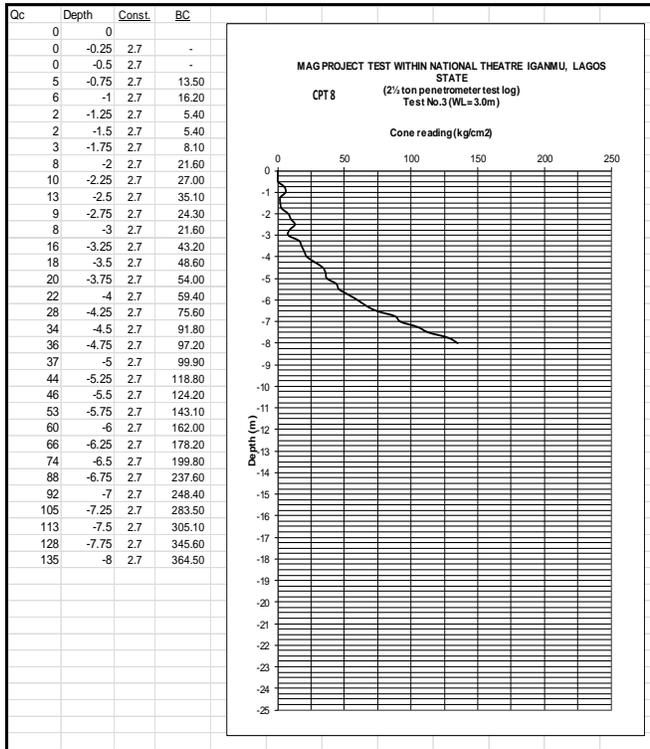
Figure 5c: Selected cone resistance versus depth curve at test point 8.
