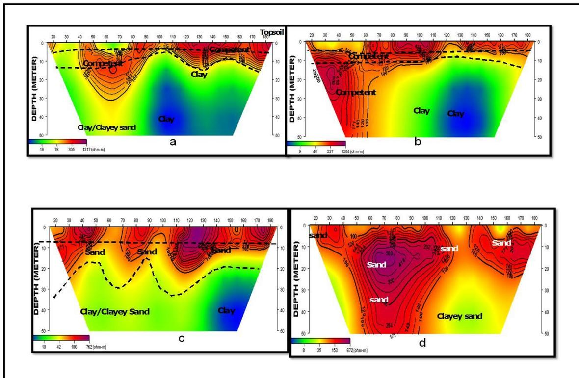
Figure 4 (a-d): 2-D resistivity sections along traverses one to four.
