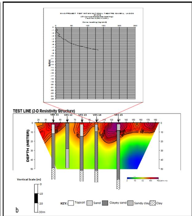
Figure 6: Correlation of the 2-D, VES and CPT Results along (a) Traverse One and (b) Traverse three.
