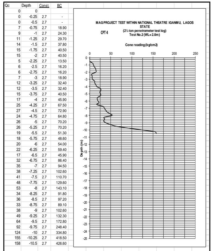
Figure 5b: Selected cone resistance versus depth curve at test point 4.
