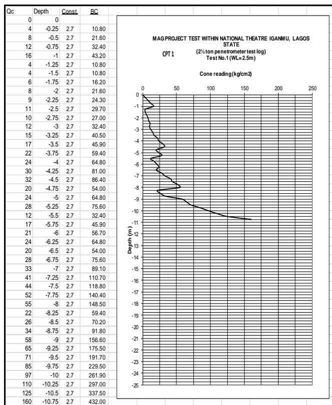
Figure 5a: Selected cone resistance versus depth curve at test point 1.
