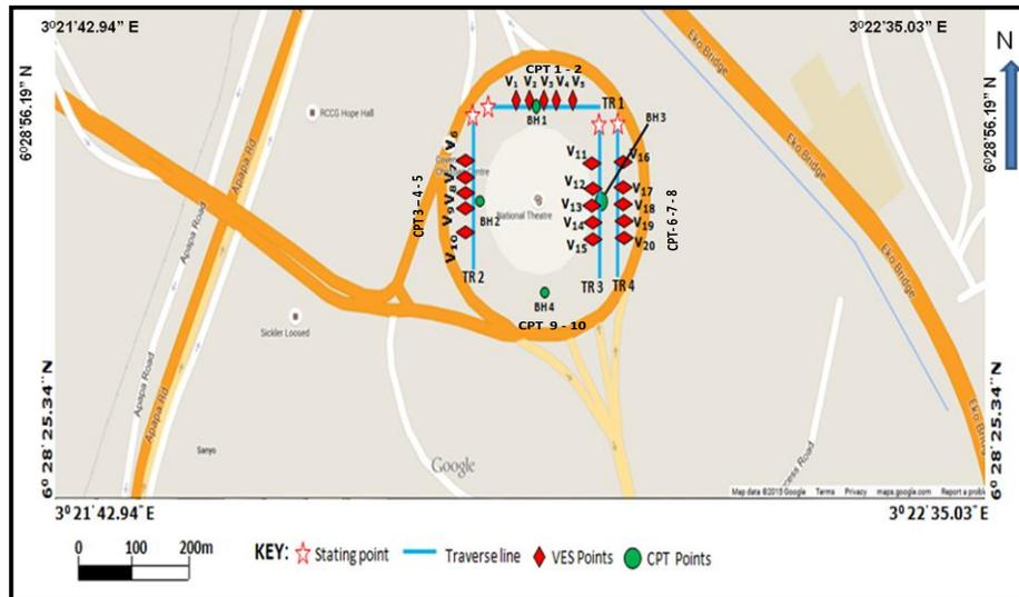
Figure 1: Map of the study area showing the electrical soundings (VES), boreholes (BH) and Cone Penetration Test (CPT) points.
