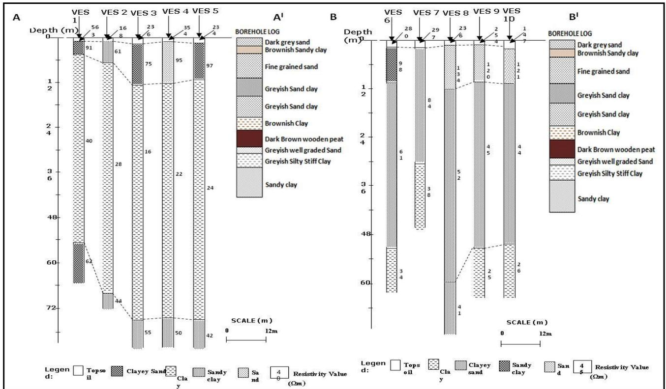
Figure 2: Geo-electric Section along AA<sup>I</sup> and BB<sup>I</sup>.
