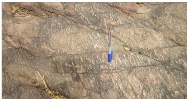
Plate 2: Mineral stretching in mylonites in a direction perpendicular to applied stress (Note that the biro is placed relative to the north direction) (N10°16.604'- E13°19.912').
