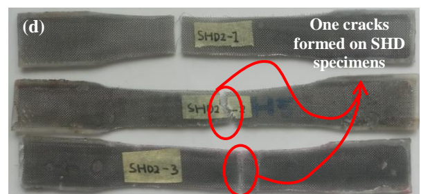
Figure 6 Failure mode of SSM composite specimens after tensile testing, a) SLD1, b) SLD2, c) SHD1, and d) SHD2
