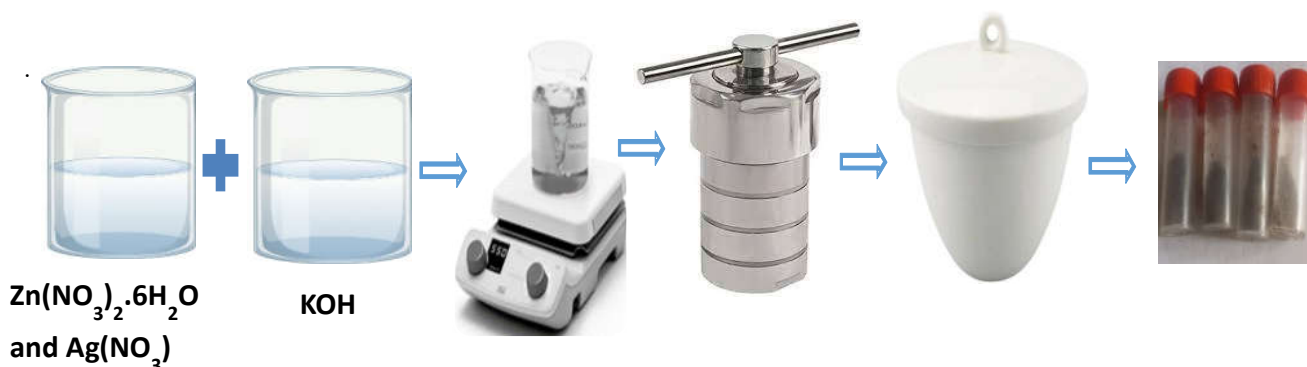
Figure 1: schematic diagram for the hydrothermal process of Ag doped zinc oxide NPs
