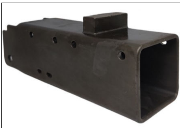
Figure 20: The actual casting product shows that casting simulation is successful in giving insight into predicting and preventing the occurrence of flaws
