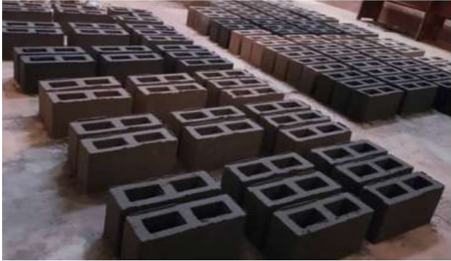
Figure 1. Freshly made hollow sandcrete blocks (Ikeagwuani et al., 2020)
