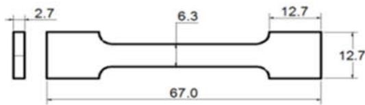
Figure 2: Dimension of Tensile bar (mm)
