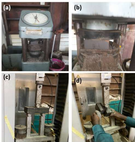
Figure 3: (a) & (c) Compressive strength and flexural strength test machines, (b) & (d) Performance of compression and flexural load-carrying capacity of bricks after failure.
