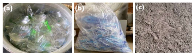
Figure 1: (a) Recycled-PET; (b) Recycled-LDPE; (c) Unilorin River sand
