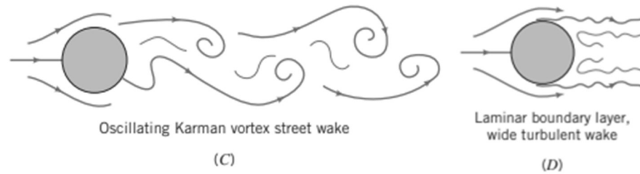
Figure 2. Flow characteristics for the Reynolds number range in this study (Munson, 2022).
