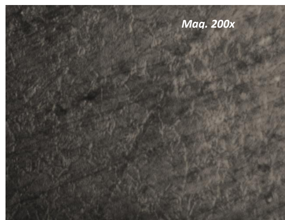
Plate 3: Microstructure of sample C showing martensite (dark region) in ferrite (grey region) matrix.
