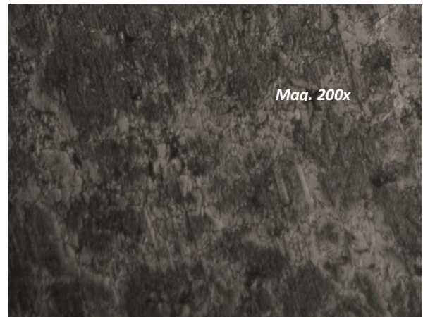
Plate 2: Microstructure of sample B showing martensite (dark region) in ferrite (grey region) matrix.
