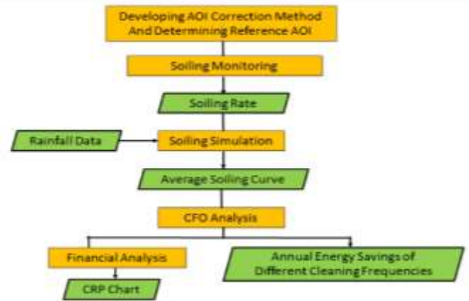
Figure 5: Methodology of the Soiling Analysis (Naeem and TamizhMani, 2015).
