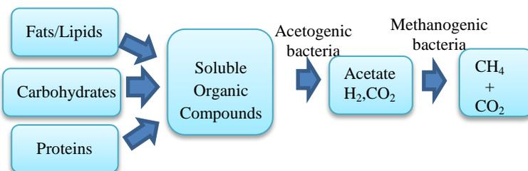
Figure 1: Schematic biochemical process stages of anaerobic digestion (Source: Achinas and Euverink, 2016)
