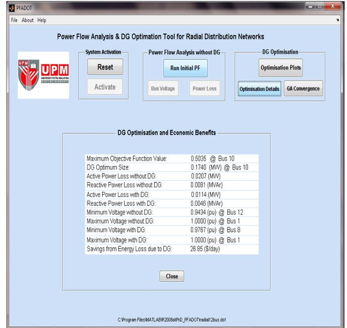
Figure 10: DG Optimisation Details of a 12-bus System.
