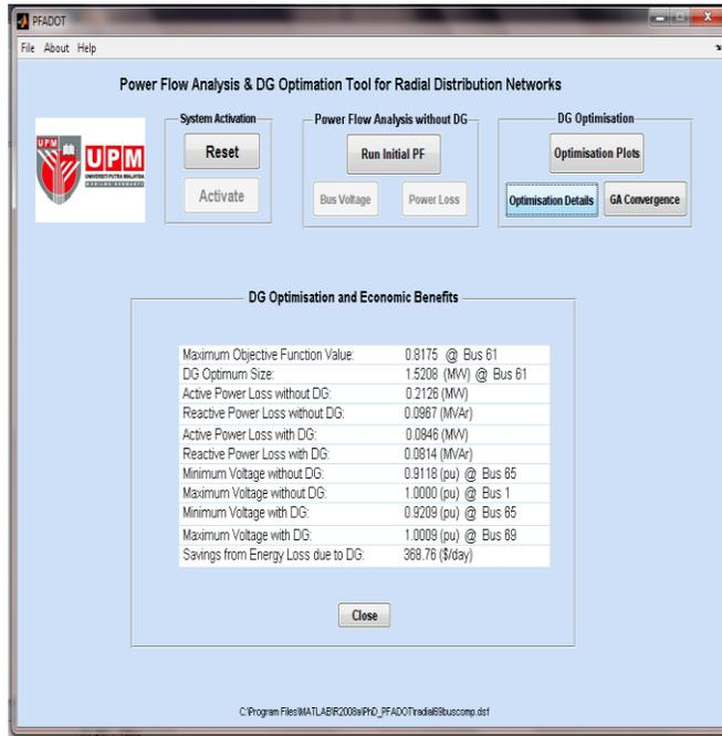
Figure 16: DG Optimisation Details for the 69-bus System with Composite Loads Models.
