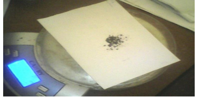
Figure 3: Electronic weighing machine for measuring the weight of the metallic contaminants.
