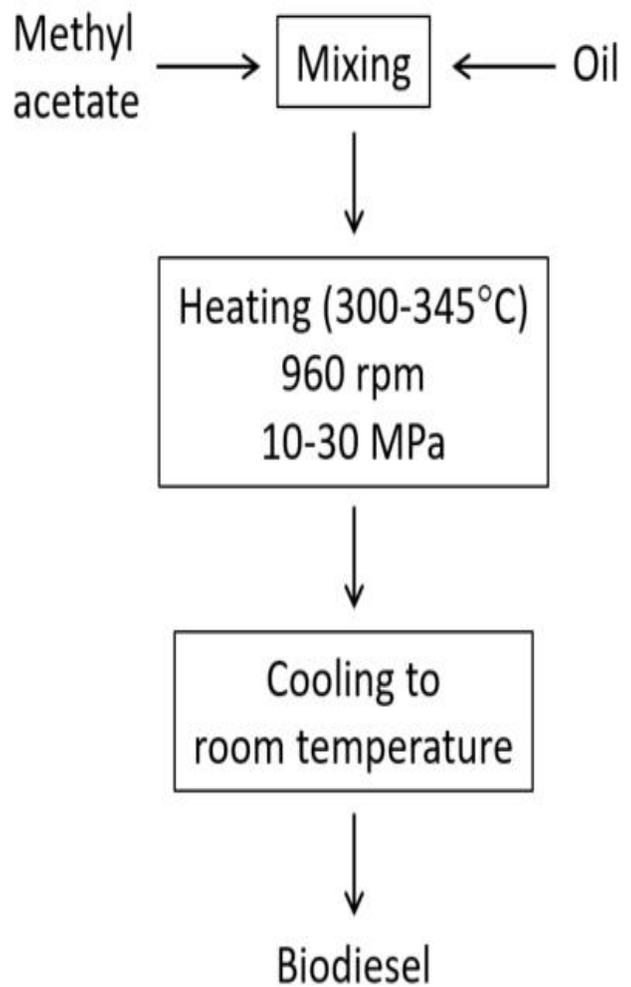
**Figure 1: Step-by-step biodiesel production via supercritical methyl acetate transesterification cycle.**
