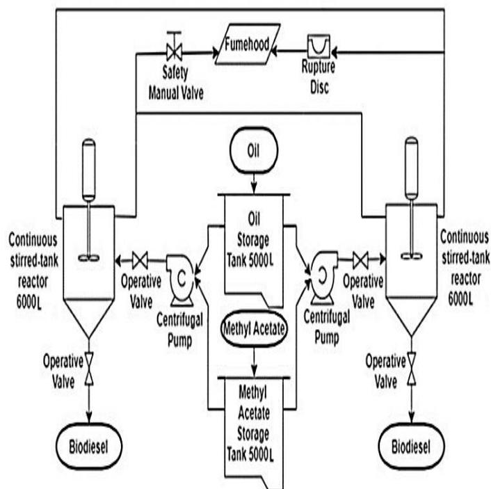
Figure 2: Illustration of the production process of biodiesel via supercritical methyl acetate transesterification method.
