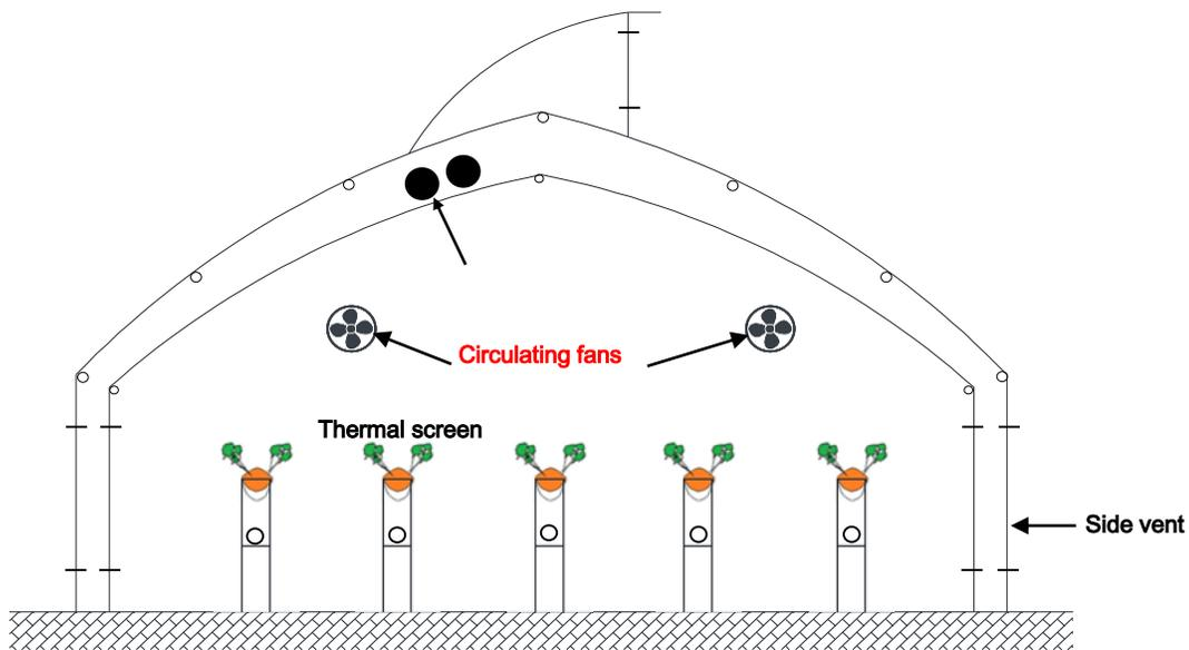
Figure 2: Q-greenhouse with a thermal screen on the north side of the greenhouse roof.
