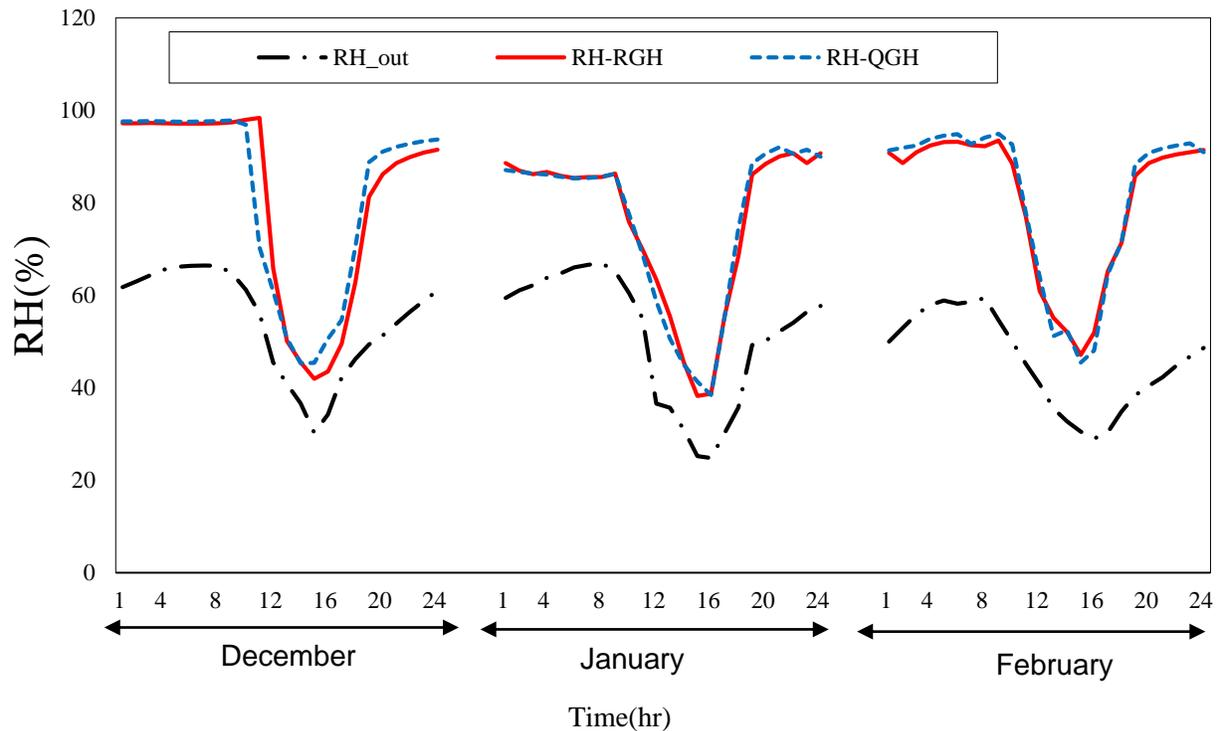
Figure 6: RH variations in the RGH, QGH and ambient.
