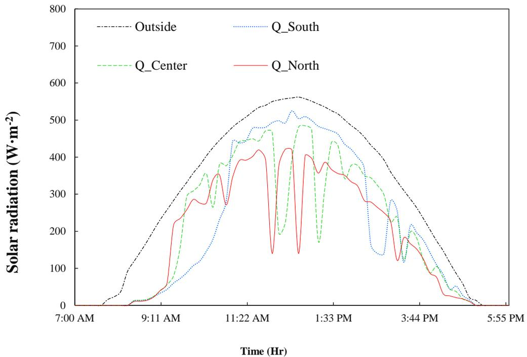
Figure 10: The trend of daily solar radiation inside vs. ambient of Q-greenhouse.
