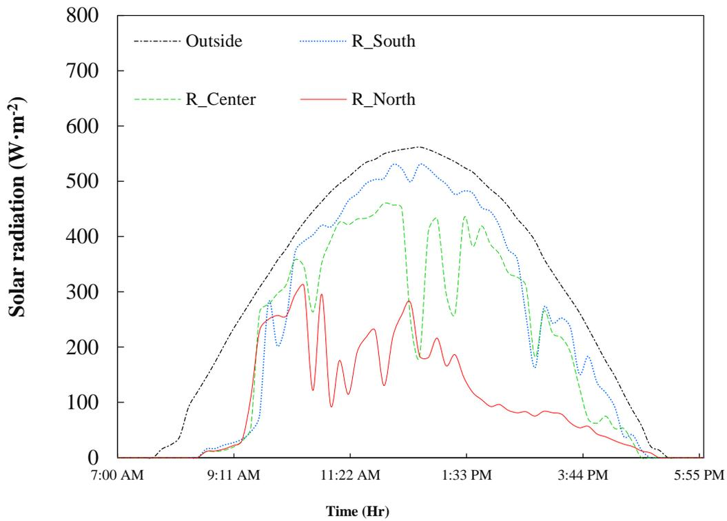
Figure 9: The trend of daily solar radiation inside vs. ambient, of R-greenhouse.
