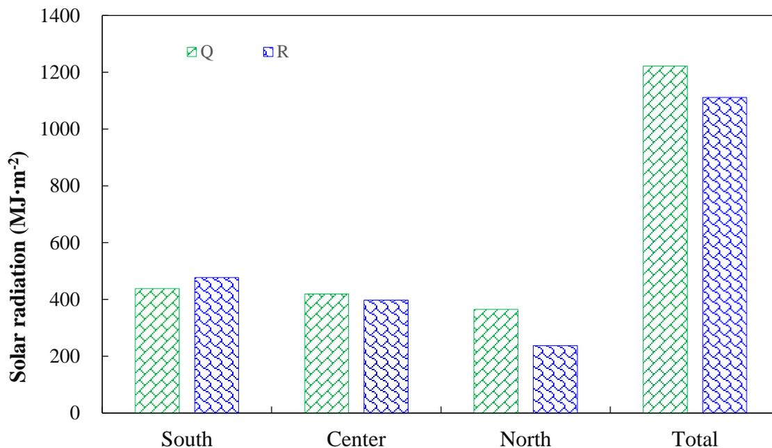
Figure 11: Total solar radiation received by R and Q greenhouses at the south, centre, and north side.
