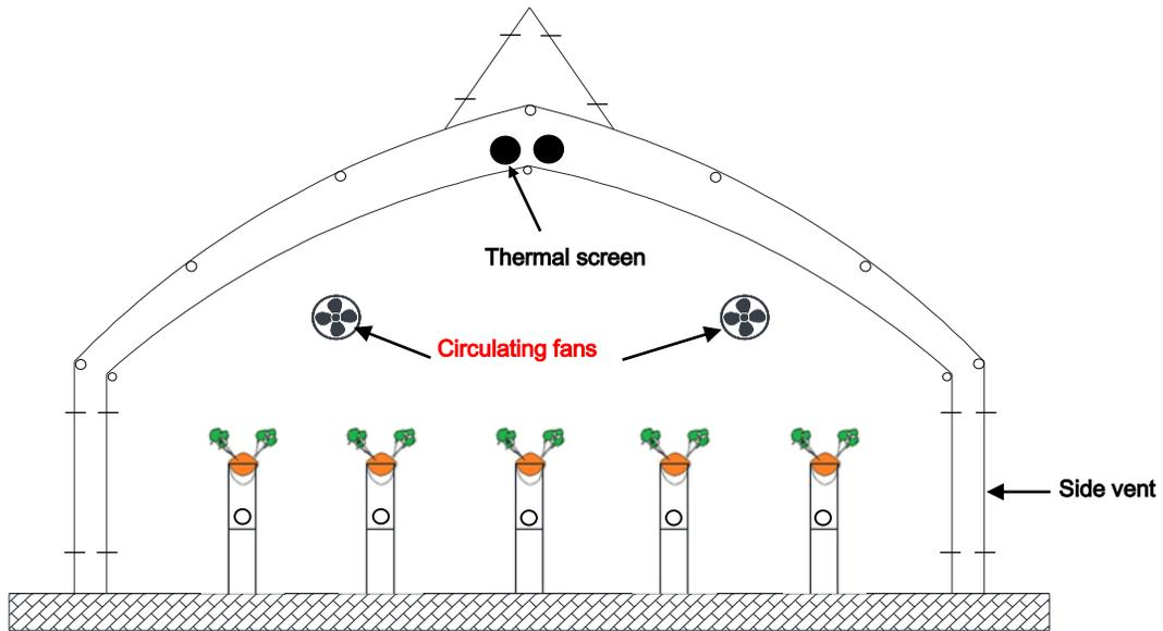
Figure 1: R-greenhouse with a thermal screen at the roof ridge.
