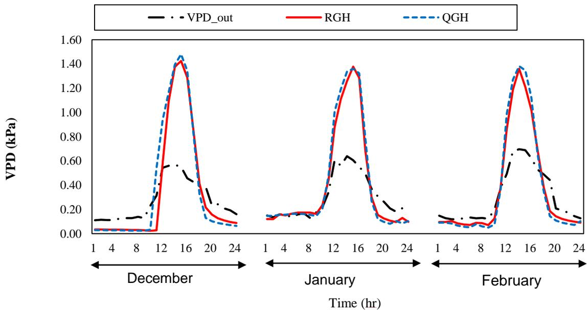
Figure 5: VPD variations in the RGH, QGH and ambient.
