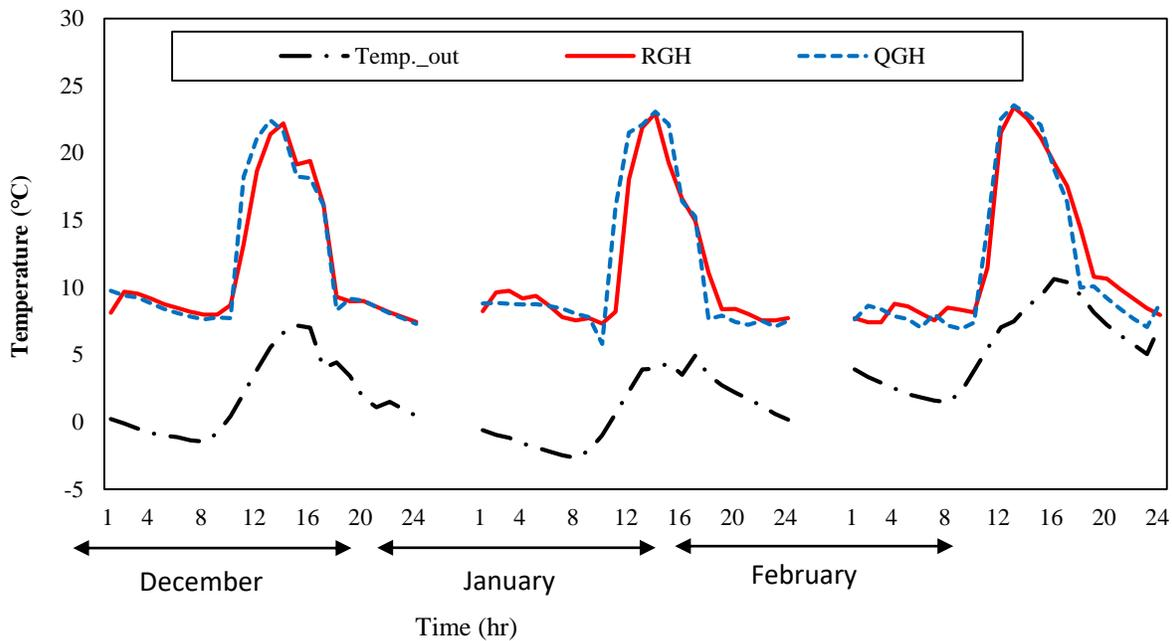
Figure 4: RGH vs QGH and their ambient temperature variations.
