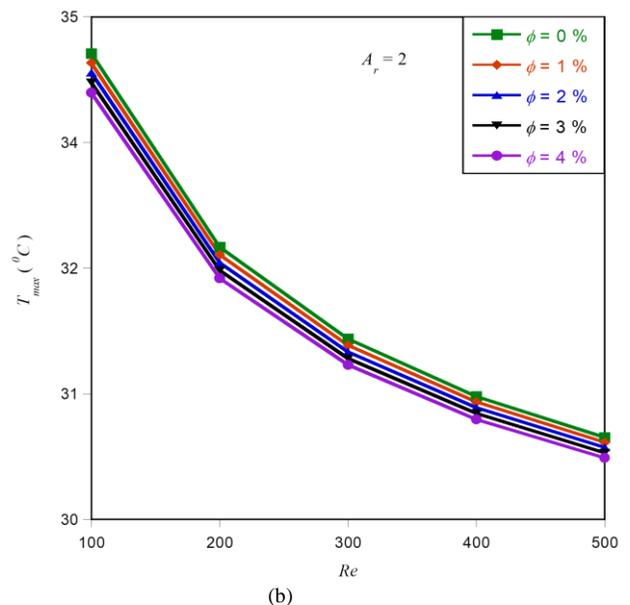
**Figure 3: Effect of (a)  $\phi$  at fixed  $Re = 500$  and different  $Ar$ , and (b)  $Re$  at fixed  $Ar = 2$  and different  $\phi$  on maximum wall temperature.**
