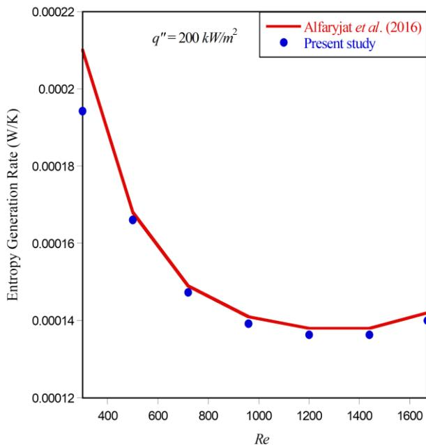
**Figure 2: Validation of the present study with the work of Alfaryjat *et al.* (2016)**
