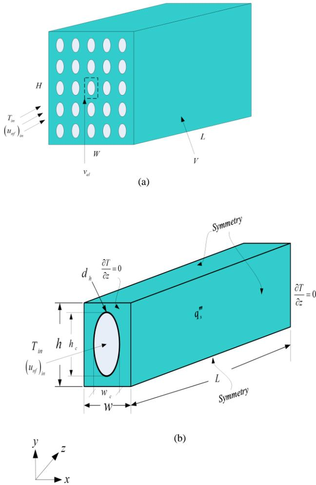
**Figure 1:** The (a) configuration of the elliptical cooling channels (b) elemental volume microchannel.
