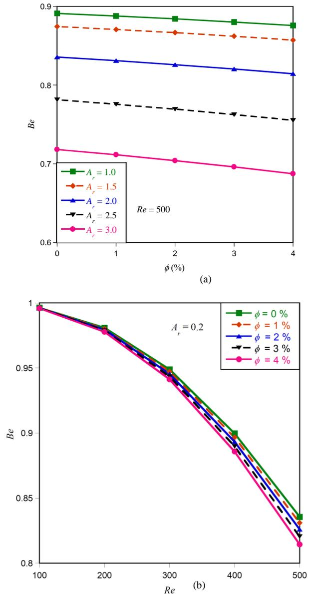
Figure 6: Effect of (a)  $\phi$  at fixed  $Re = 500$  and different  $A_r$  and (b)  $Re$  at fixed  $A_r = 2$  and different  $\phi$  on  $Be$ .
