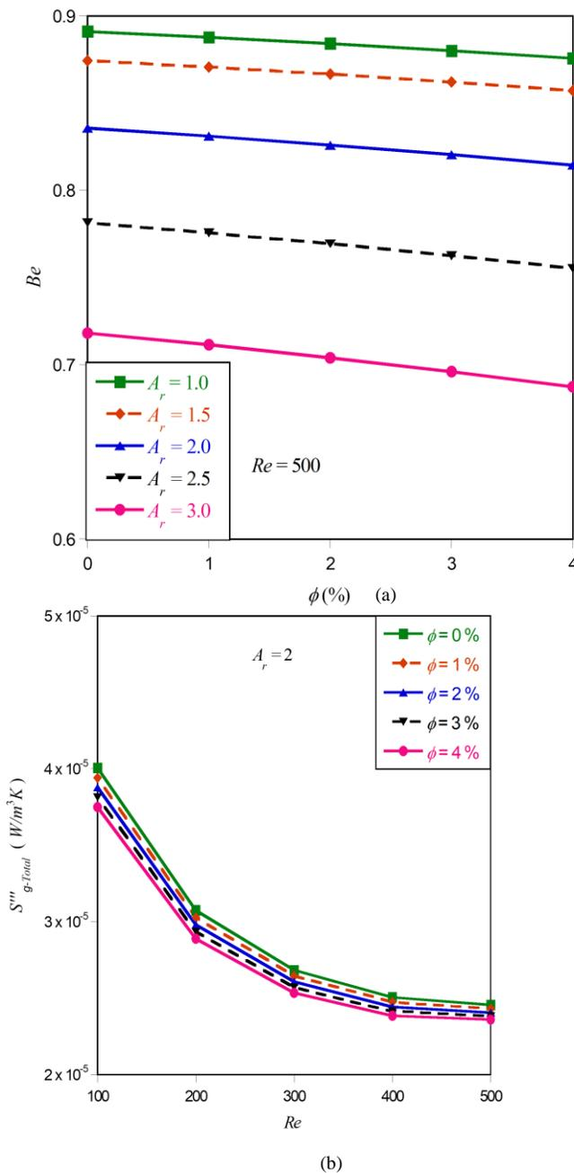
Figure 7: Effect of  $Re$  on (a)  $\dot{S}'''_{g-th}$  and  $\dot{S}'''_{g-fr}$  at fixed  $A_r = 2$  and different  $\phi$  and (b)  $Re$  on total  $\dot{S}'''_{g-Total}$  at fixed  $A_r = 2$  and different  $\phi$
