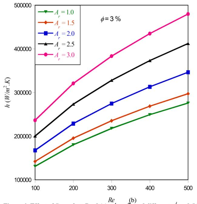
**Figure 4: Effect of  $Re$  on  $h$  at fixed (a)  $A_r = 2$  and different  $\phi$  and (b)  $\phi = 3\%$  and different  $A_r$**
