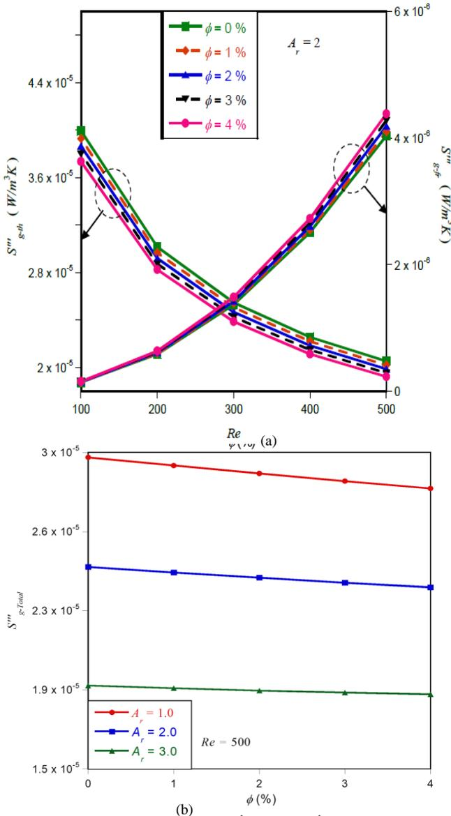
**Figure 5: Effect of  $\phi$  on (a)  $\dot{S}'''_{g-th}$  and  $\dot{S}'''_{g-fr}$  and (b)  $\dot{S}'''_{g-Total}$  at different  $A_r$  and fixed  $Re = 500$ .**
