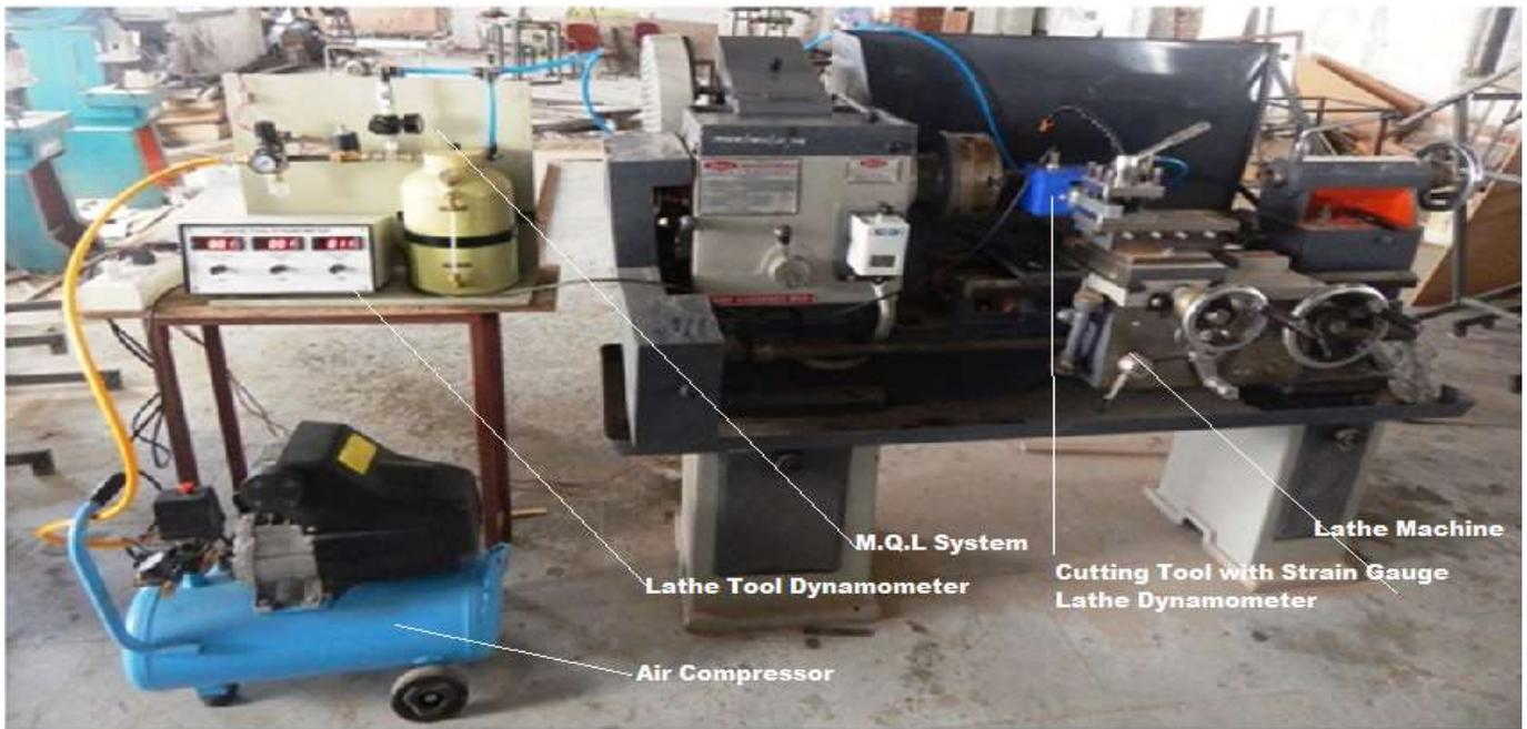
Figure 1(a): Experimental Setup.
