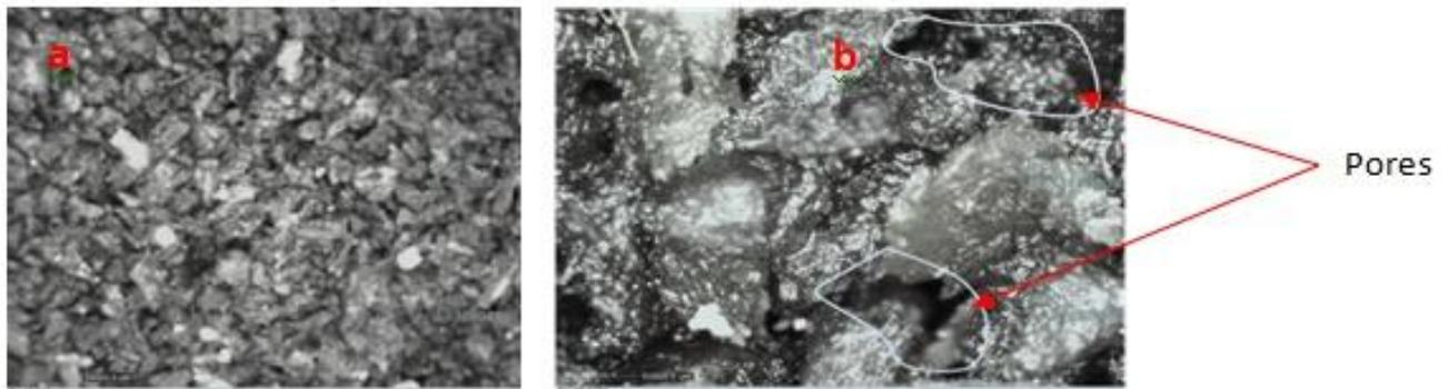
Figure 3: Optical micrograph of the abrasive sandpaper for 250  $\mu\text{m}$  grain size: Magnification (a) 50X and (b) 250X.
