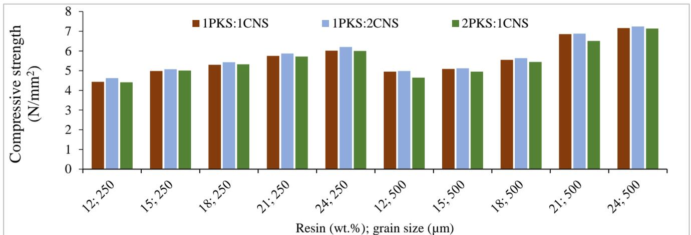
Figure 7: The variation effects of grain size, mixing ratio and resin weight percent on compressive strength.
