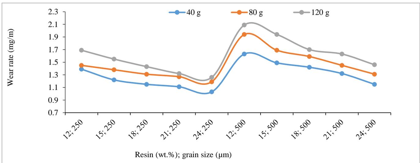
Figure 9: The variation effects of grain size and resin weight percent on wear rate at 150 °C.
