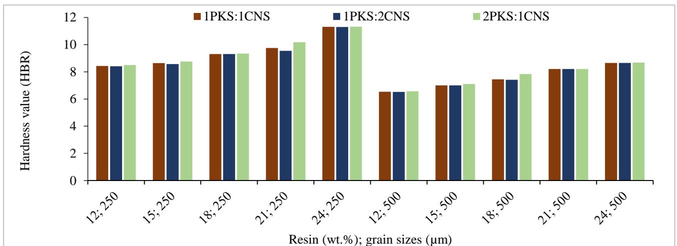
Figure 6: The variation effects of grain size, mixing ratio and resin weight percent on the hardness.
