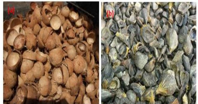
**Figure 1: Raw samples of (a) Coconut shells and (b) Palm kernel shells**
