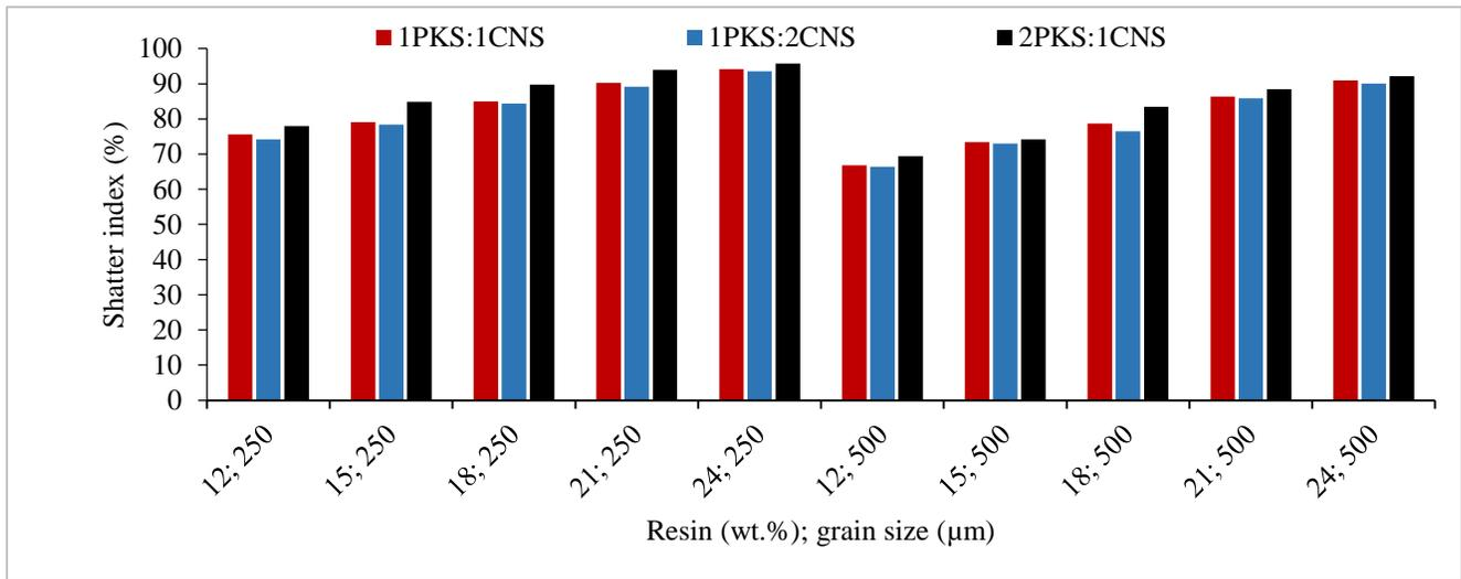
Figure 5: The variation effects of grain size, mixing ratio and resin weight percent on shatter index.
