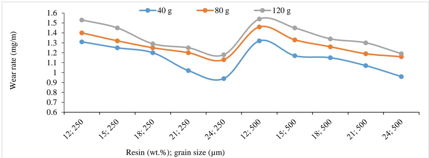
Figure 8: The variation effects of grain size and resin weight percent on wear rate at 50 °C.
