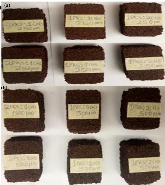
**Figure 2: Abrasive samples of (a) 250 μm grain sizes and (b) 500 μm grain sizes**
