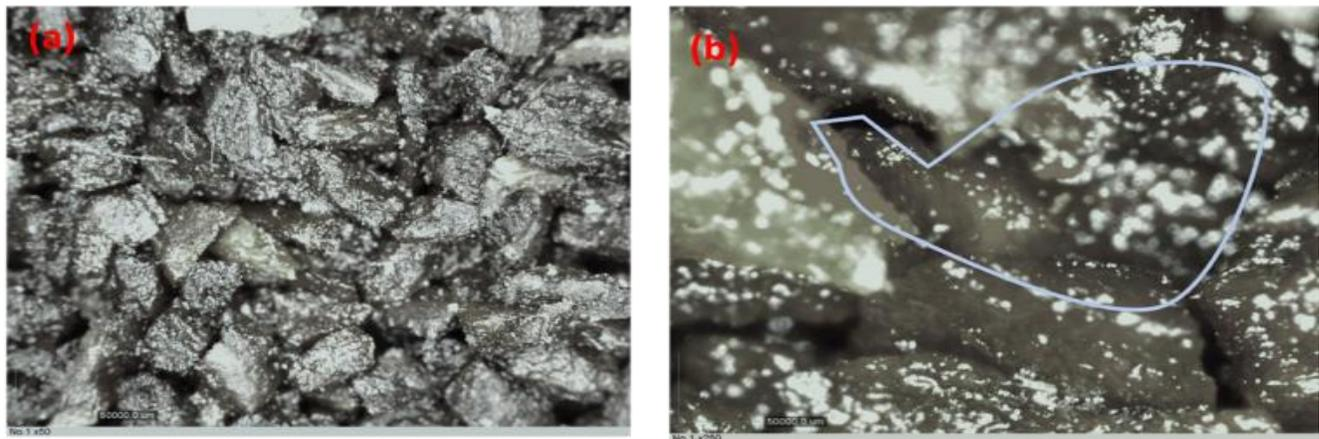
Figure 4: Optical micrograph of the abrasive sandpaper for 500 μm particle size: Magnification (a) 50X and (b) 250X.
