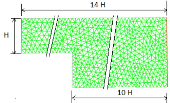
Figure 3: Backward facing step domain and mesh.
