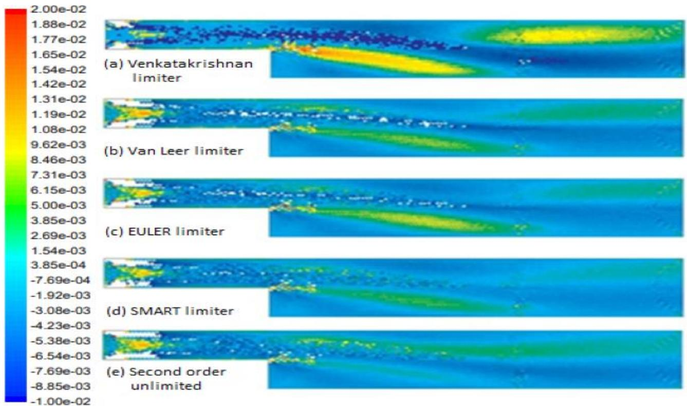
Figure 4. Effect of flux limiters on x-velocity error. The error was calculated as the difference between the reference solution and the test solution.
