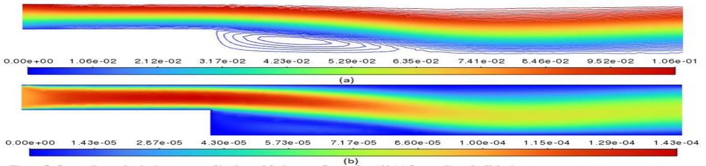
Figure 5. Streamline and velocity contour of backward facing step flow at Re=100 (a) Stream line; (b) Velocity contour.
