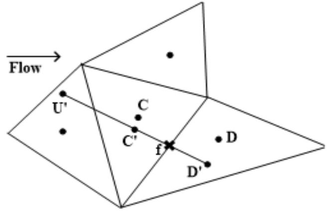
Figure 2: Spatially corrected cell centres and fictitious cell.
