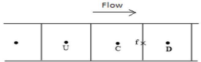
Figure 1: Upwind and downwind cell of one-dimensional mesh.
