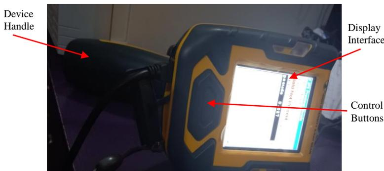
Figure 5: Metal Analyzer model no Niton XL2 by Thermo scientific.
